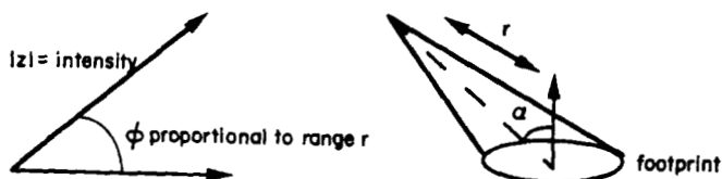
Figure 2. Model of (range, intensity) pair as complex number
