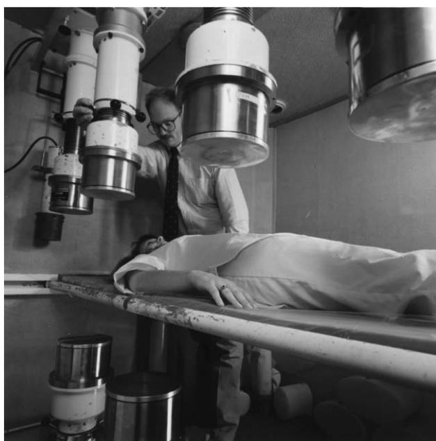
**Fig. 2** Inside the Harwell Laboratory shielded, whole-body monitor showing the positions of the six NaI crystal  $\gamma$ -detectors that will be aligned above and below the supine subject.
