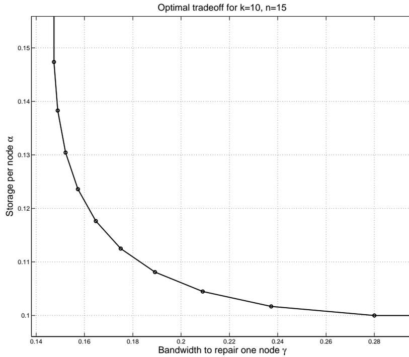
Fig. 4. Optimal tradeoff curve between storage  $\alpha$  and repair bandwidth  $\gamma$ , for  $k = 5, n = 10$  (left) and  $k = 10, n = 15$  (right). For both plots  $\mathcal{M} = 1$  and  $d = n - 1$ . Note that traditional erasure coding corresponds to the points  $(\gamma = 1, \alpha = 0.2)$  and  $(\gamma = 1, \alpha = 0.1)$  for the top and bottom plots.
