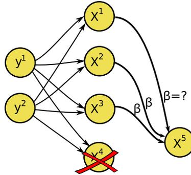
Fig. 1. The repair problem: Assume that a  $(4,2)$  MDS erasure code is used to generate 4 fragments (stored in nodes  $x^1, \dots, x^4$ ) with the property that any 2 can be used to reconstruct the original data  $y^1, y^2$ . When node  $x^4$  fails, and a newcomer  $x^5$  needs to generate an erasure fragment from  $x^1, \dots, x^3$ , what is the minimum amount of information that needs to be communicated?
