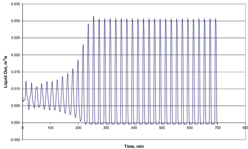
**Figure 8, Severe Slugging Phase Portrait – 1000m Riser, GOR 107  $\text{sm}^3/\text{sm}^3$**
