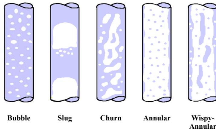
The identification and classification of flows into flow patterns, while subjective, has presented a useful approach for the modelling of multiphase flows. In particular, the pressure drop and phase holdups differ significantly from one pattern to another and hence the prediction of multiphase flows benefits from a knowledge of the flow pattern and the subsequent application of appropriate relationships specific to the flow pattern in question.
