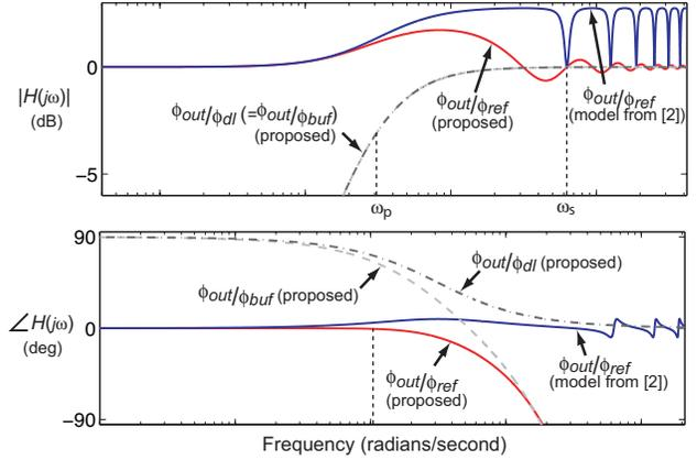
Fig. 3: Frequency response of a first order charge-pump DLL using the proposed model and the z-domain model from [2].
