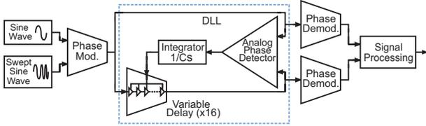
Fig. 4: Simplified functional model of first order analog DLL.
