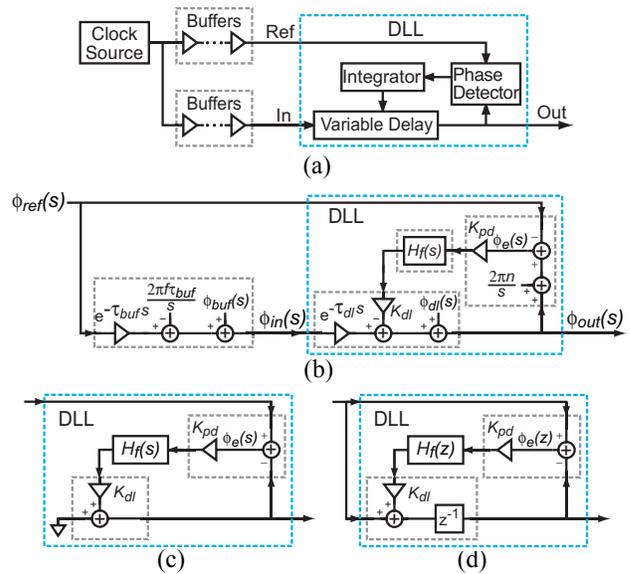
Fig. 1: (a) Basic delay-locked loop architecture with system interconnections and different linearized models of system: (b) proposed model (c) model from [1] (d) model from [2].
