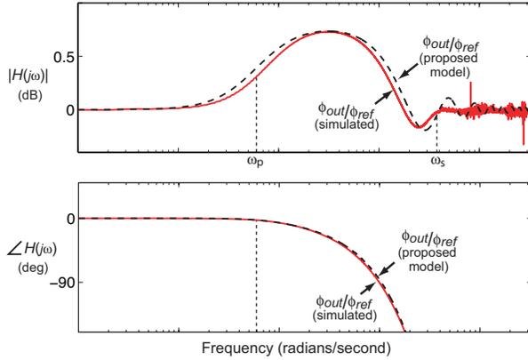
Fig. 5: Calculated and simulated frequency response of first order DLL with analog (multiplying) phase detector ( $\omega_p = \omega_s / 62.8$ ).
