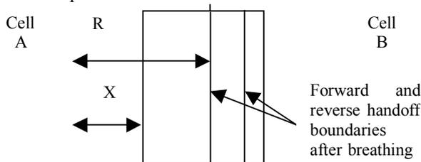
**Figure 2. Handoff boundary has moved closer to cell A due to loading on cell A**
