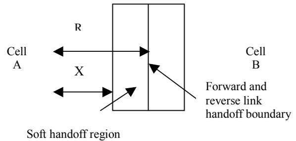
Figure 1. A balanced forward and reverse link handoff boundary case for two cells A and B
