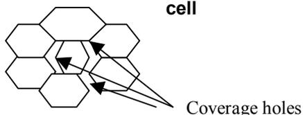
**Figure 3b. Coverage holes develop when all cells are heavily loaded**
