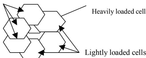
**Figure 3a. No coverage holes develop when lightly loaded cells surround a heavily loaded cell**
