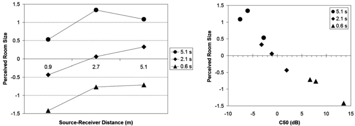
Figure 4: Results of Experiment II, in terms of source-receiver distance and reverberation time shown in the left chart. The right chart shows the relationship between  $C_{50}$  and perceived room size.
