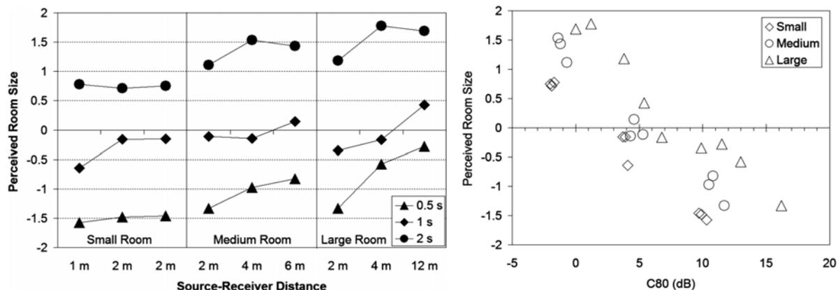
Figure 2: Results of Experiment I, showing subjective ratings in terms of source-receiver distance, reverberation time, and room volume on the left chart. The relationship between  $C_{80}$  and perceived room size is shown on the right, with data for the three room volumes separated.
