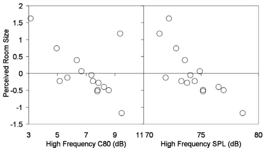
Figure 8: Results of Experiment III, in terms of  $C_{80}$  and stimulus sound pressure level at high frequencies (combined 2 kHz and 4 kHz octave band measurements).
