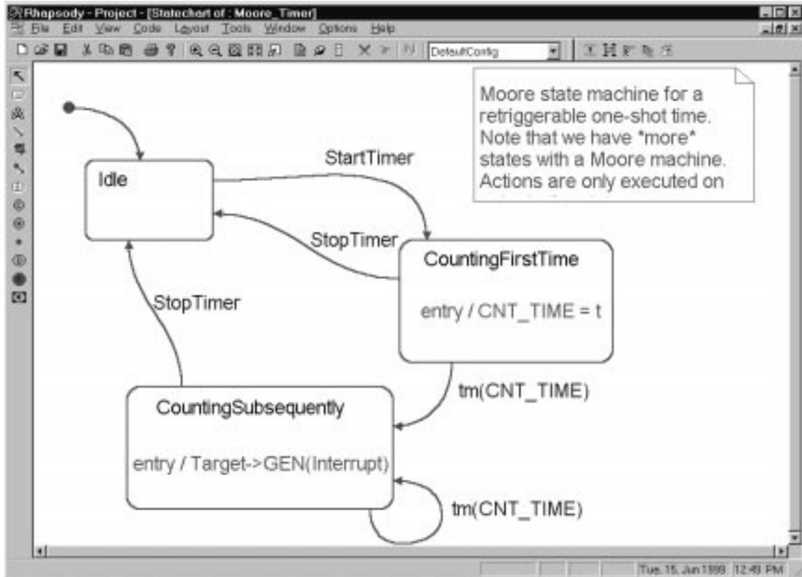
You can see that an additional state is needed since the actions performed during the Counting Down state differ from the actions performed on subsequent timer restarts.
