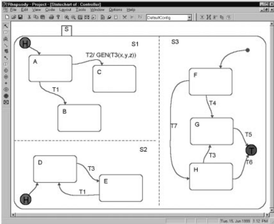
Concurrency in statecharts is shown using dashed lines, as shown above. The overall state being modeled is S, and is broken up into three distinct, concurrent state machines, S1, S2, and S3. Each of these is an independent state machine with its own initial state, history, and behavior. In such a concurrent system it is important to note that *while in S, the system is in one state each from S1, S2, and S3 at the same time.*
