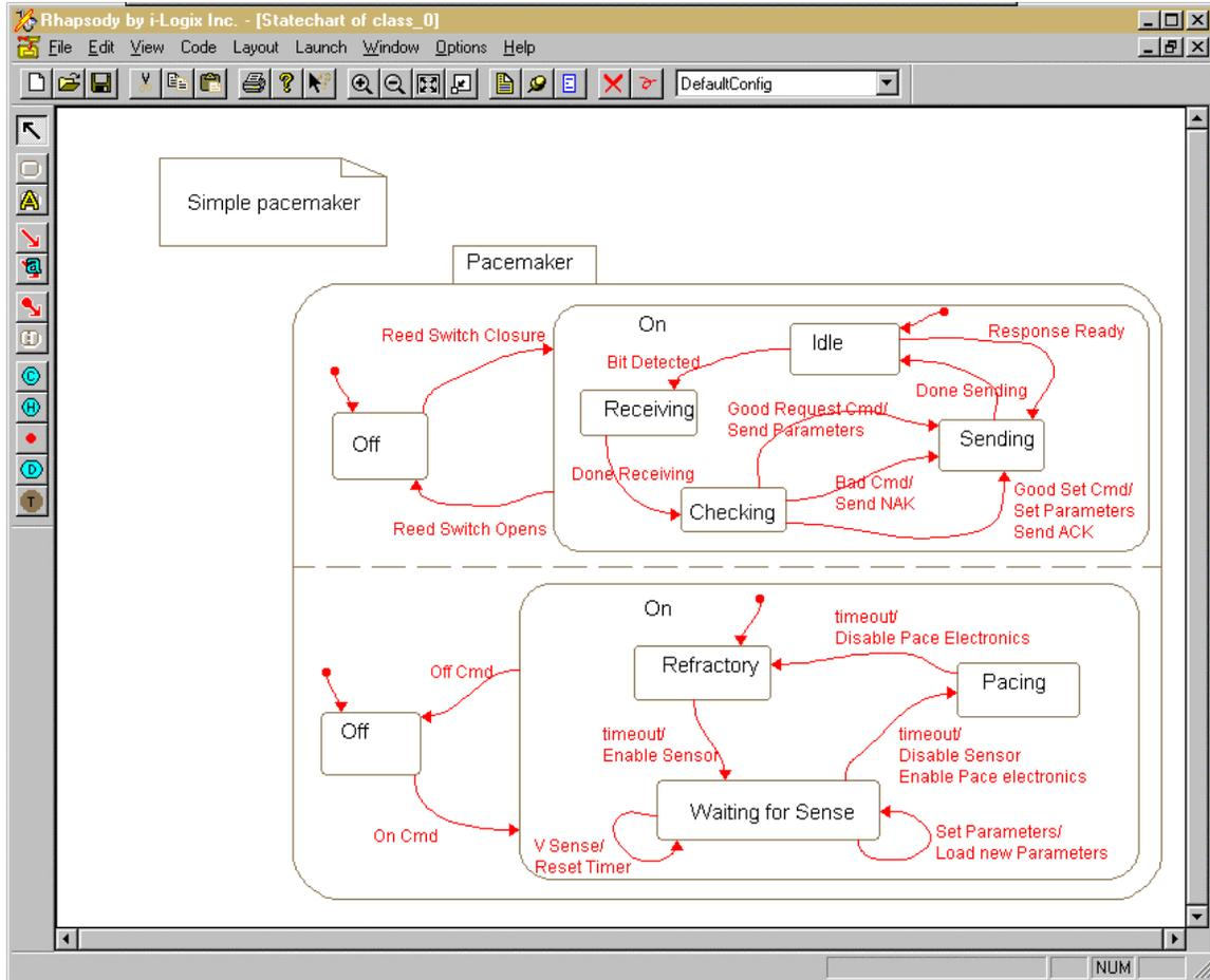
Note that the communications system is an FSM which operates concurrently with the pacing engine. It would be inappropriate to disable pacing while communication occurs. The two FSMs are synchronized by the Set Parameters transition. It is initiated by the Good Set Cmd received by the communications subsystem, and results in a propagated transition Set Parameters in the pacing FSM.
