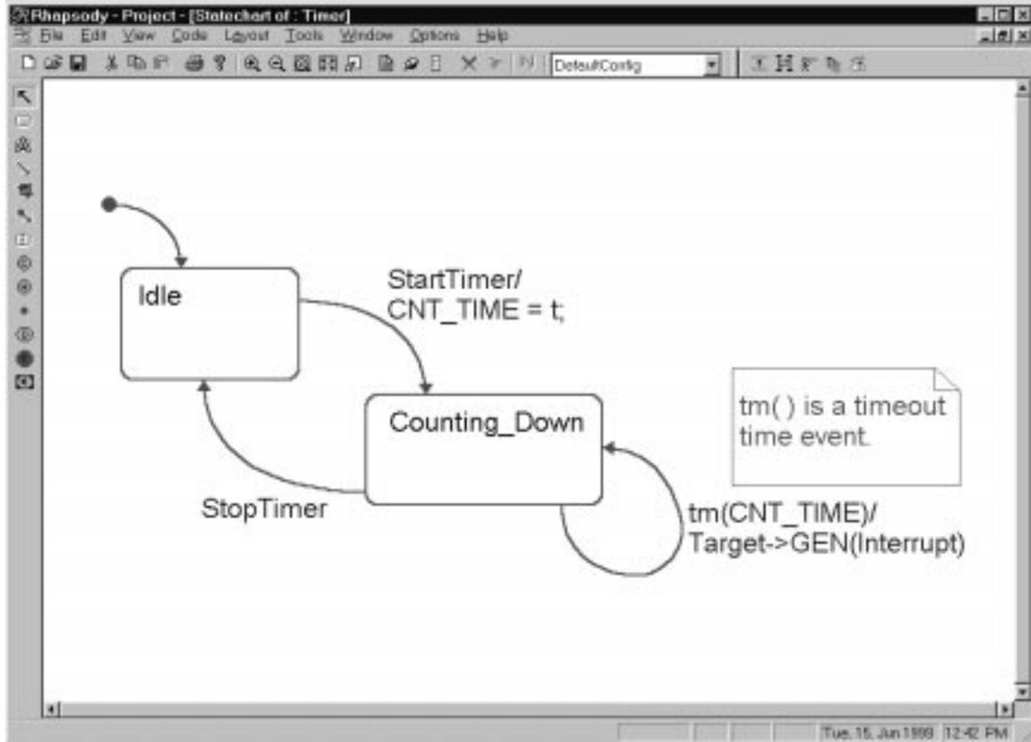
States here are shown as rounded rectangles. Transitions are directed lines beginning at the starting state for the transitions and finishing at the target state. Transitions here have names optionally followed by actions (i.e. functions or operations) executed when the transition is taken.
