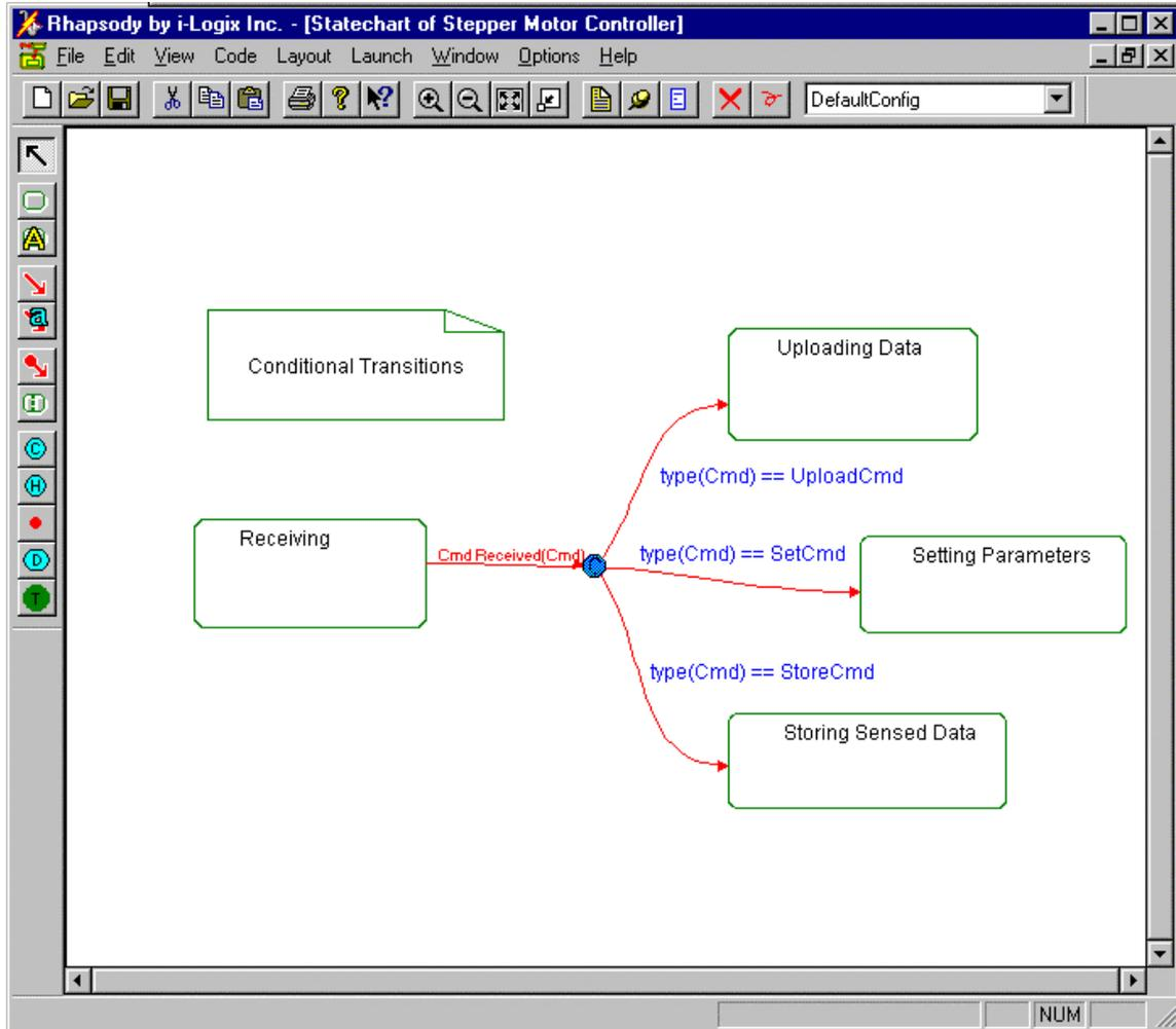
Guards are conditions which must be met for the transition to be taken even when the event causing the transition has occurred. Guards are shown in square brackets to distinguish them from event data (which is shown in parentheses). A common guard is that some other concurrent state machine must be in a certain state. This is normally shown as `[in(G)]` indicating that the other state machine must be in state G for the transition to be taken.
