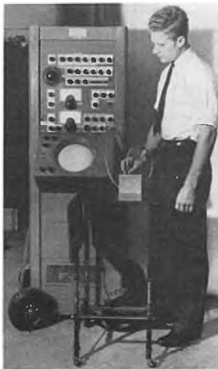
FIG. 2a. Type A supersonic reflectoscope.
