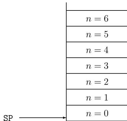
This is an imagined snapshot of the stack during execution of the innermost recursive call, i.e. `fact 0`. All the local variables for the upper stages are stacked up above, with each instance of the function having its own stack frame, and when the calls are finished the stack pointer `SP` moves back up.
