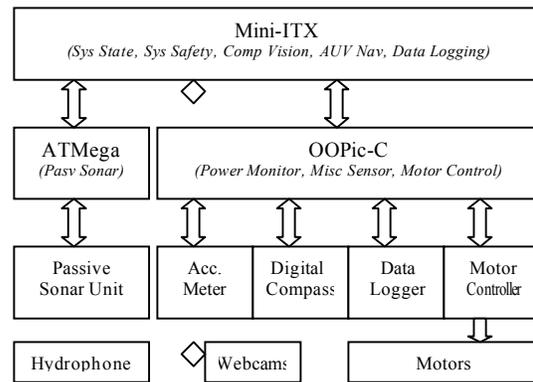
Figure 6. PPU & SPU Control System Architecture – Software Agents in Parenthesis
