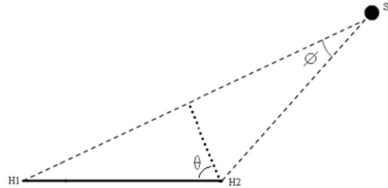
Figure 11. Conceptual representation of hydrophones in a USBL configuration on and AUV and an acoustic source.
