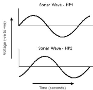
Figure 12. Analog Sonar AC waves as received on the hydrophones.
