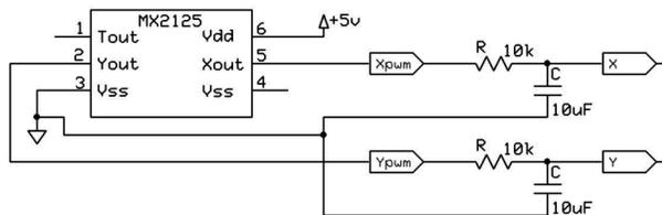
Figure 7. Accelerometer PWM signal to Analog Signal R-C Converter
