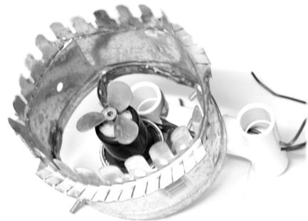
Figure 4. Bilge pump based thruster design.
