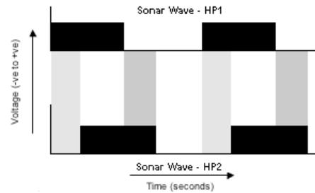
Figure 13. AC Sonar waves converted to equivalent TTL.
