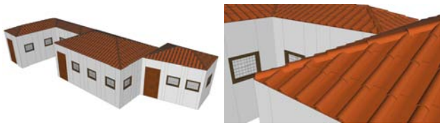
Figure 13: Left: The simple grammar is applied to three different footprints. Please note how the occlusion query avoids placing windows at the intersection of two neighboring buildings. Right: The roof is modeled by bricks on the roof planes and the roof edges.
