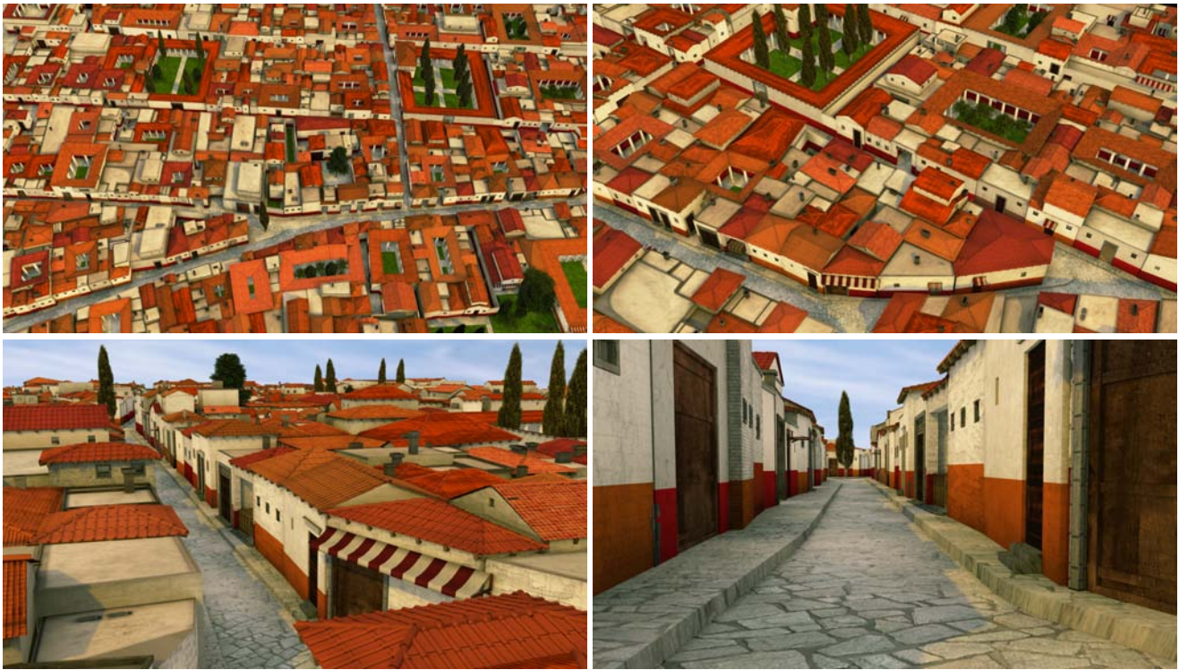
Figure 18: Various views of the procedural Pompeii model. Based on real building footprints, the city was generated with 190 manually written CGA shape rules. Hence, the whole model is a rule-based composition of 36 terminal objects (plus 4 tree types and the environment).
