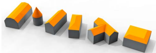
Figure 7: Selected roof types. From left to right: gambrel, cone, gabled, hipped, cross-gable, mansard.
