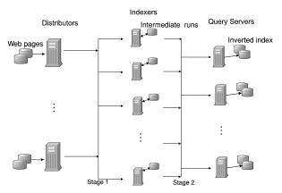
Fig. 1. Testbed architecture.
