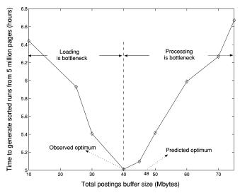
Fig. 4. Optimal buffer size.
