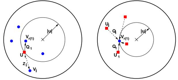
Figure 2: An illustration of random variables used in the proof: sender location  $U_1$ , receiver location  $V_{r(1)}$ , received signal power  $Q_1$ , scaled distance to random receiver  $Z_i$ , and scaled interfering sender distance  $Q_i$ .
