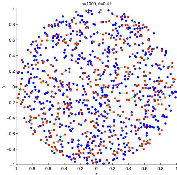
Figure 3: An example of a random topology with  $n = 1000$  nodes, for sender density  $\theta = 0.41$ . Senders are depicted as red squares, receivers as blue circles. A line connects each sender to its closest receiver.
