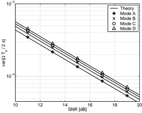
Fig. 5. Tracking variance, AWGN channel, robustness modes A-D.
