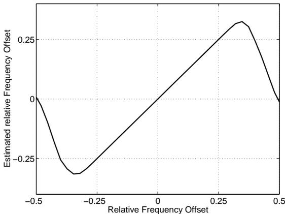
Fig. 4. Characteristic curve of frequency tracking unit.
