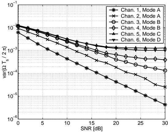
Fig. 6. Simulated tracking variance for all channels.
