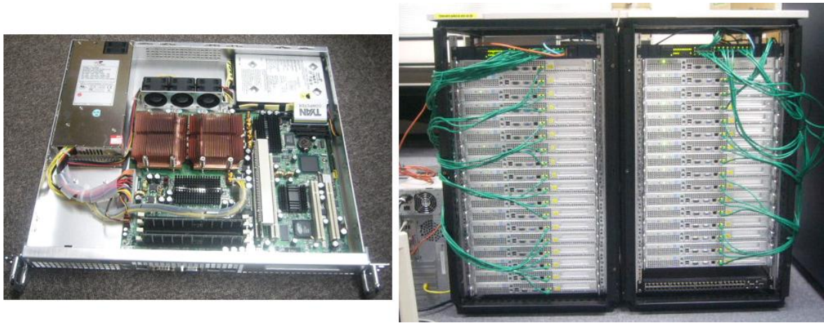
Figure 5. Photographs of a node computer having two processors and the 34-node PC cluster called FireCore.
