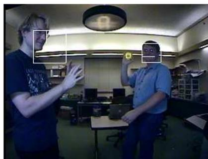
Figure 2: The visual processing step finds faces, their orientation (indicated by the small vertical or horizontal lines), and the ball (center-right).
