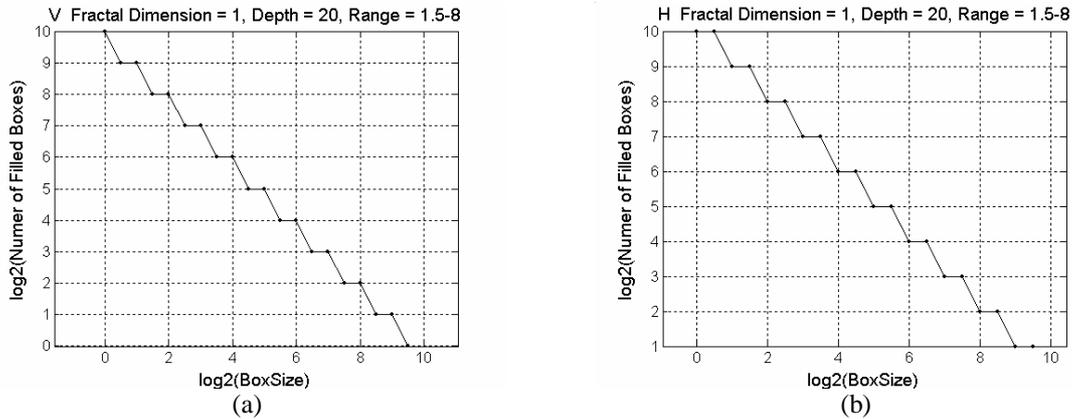
**Fig. 2.** Log-log plot of the dependence between the number of filled boxes and the box size for the linear signals shown in Fig 1. The vertical line in Fig. 1a generates the plot in Fig. 2 a, while all other lines give the diagram in Fig. 2 b. For all the instances the fractal dimension results one as expected.
