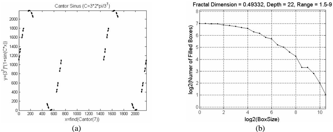
**Fig. 3.** (a) Cantor sinus signal obtained by selecting a Cantor subset of points from the discrete curve of a sinus extended over three periods. (b) Log-log plot of the dependence between the number of filled boxes and the box size for the signal shown in Fig. 3 a.
