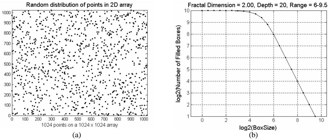
**Fig. 4.** (a) Random signal comprising 1024 points embedded in an 1024 x 1024 background array. (b) Log-log plot of the dependence between the number of filled boxes and the box size for the signal shown in Fig. 4 a.
