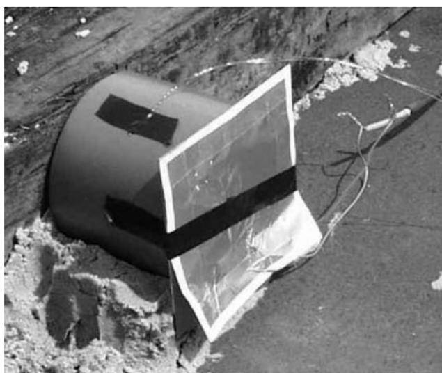
**Figure 4.** Pseudo-mine with instrumentation
