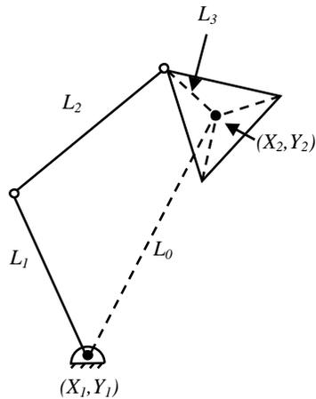
Figure 2. Example RRR kinematic chain
