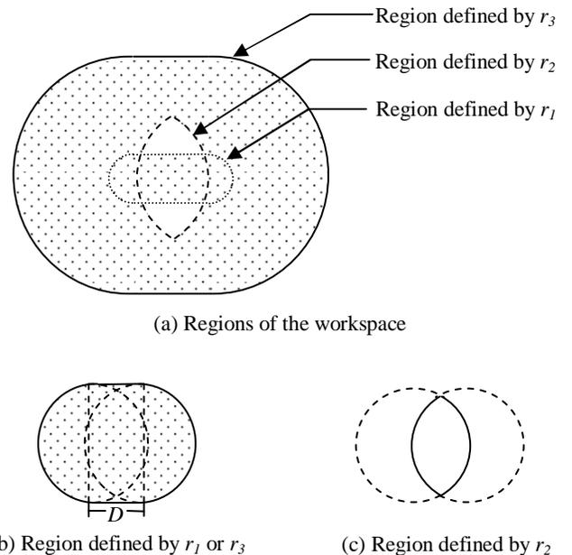
Figure 5. Shapes of regions of the workspace of a PRRR kinematic chain
