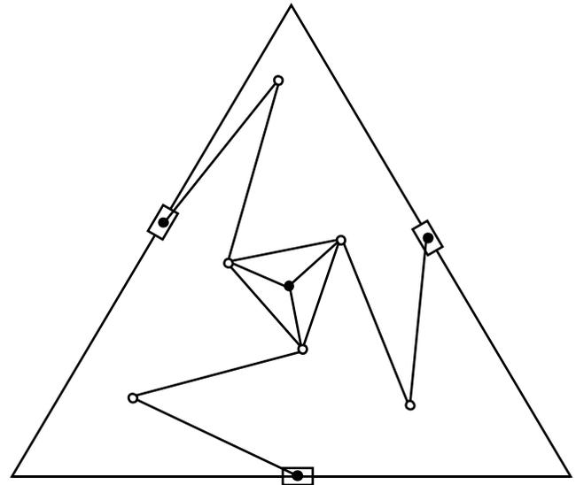
Figure 1. Example 3-PRRR planar parallel manipulator
