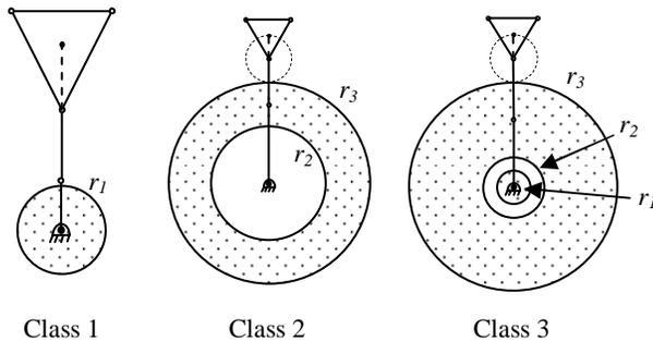
Figure 3. The 3 classes of workspaces of RRR kinematic chains
