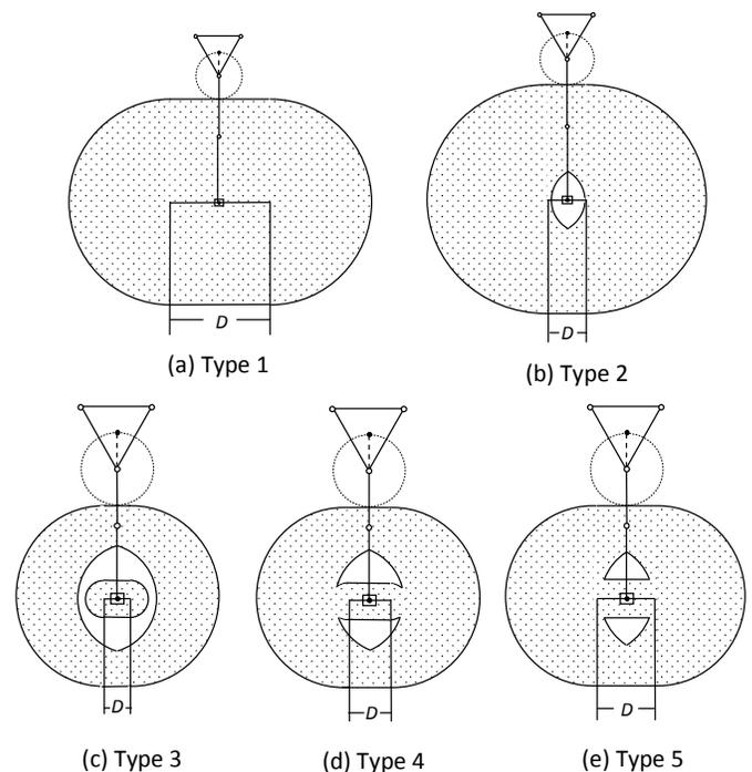
Figure 4. The 5 types of workspaces of PRRR kinematic chains
