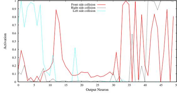
**Fig. 6.** Activation of the output neurons for bumper states at the last step of LTP
