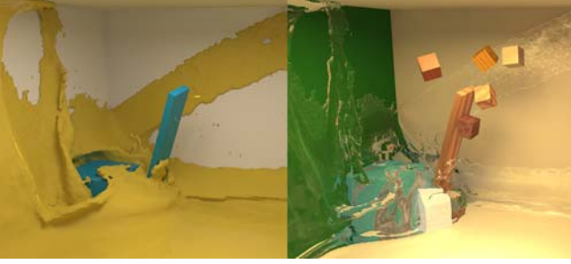
Figure 4: The left side of this figure is the computational domain, and the right is the rendered frame. On the left the yellow area is the fluid domain \mathbb{F} ; the blue is the rigid body domain \mathbb{R} . Notice that the small blocks on the right are not touching liquid, so they will be controlled by the rigid body solver until they touch liquid.
