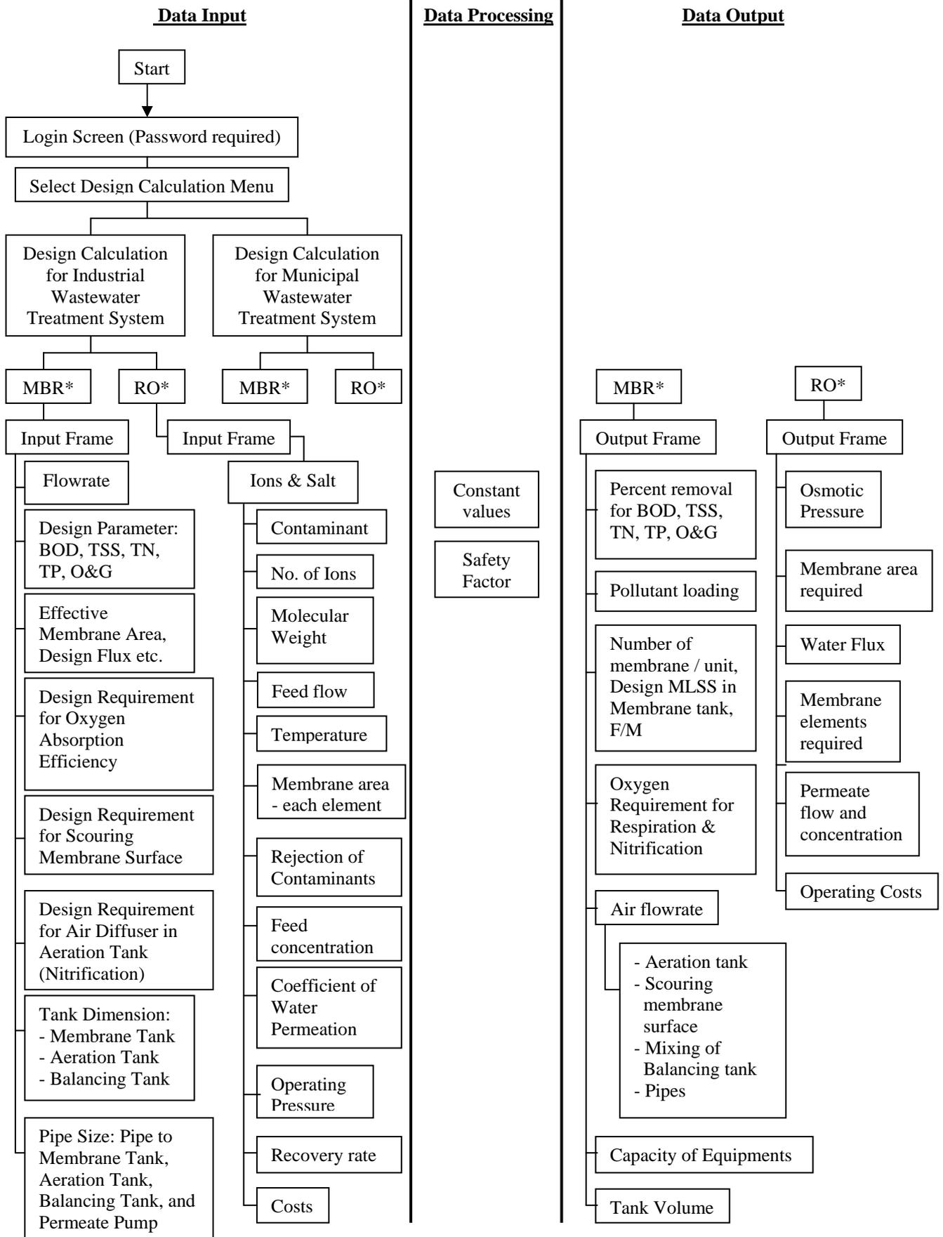
Figure 1. Architecture of WASDA – MBR and RO modules (Design Calculation Worksheet)
