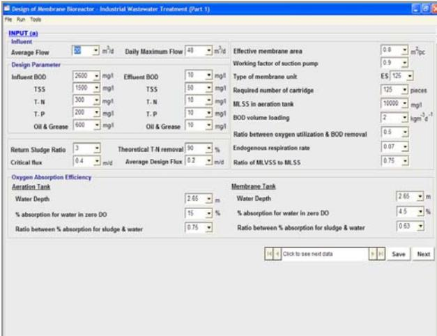
Figure 6. Input Screen for MBR module – Part 1.
