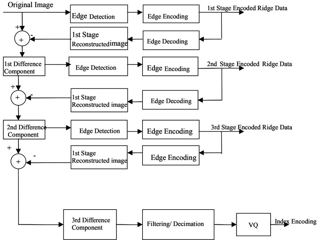
Figure 3. The overall proposed edge-detection encoding scheme for progressive image transmission.
