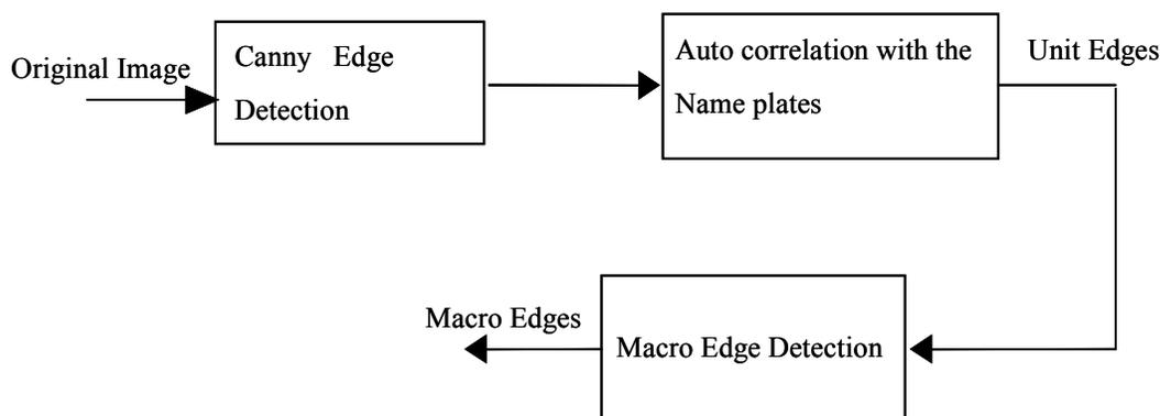
Figure 1. The unit edge detection process.
