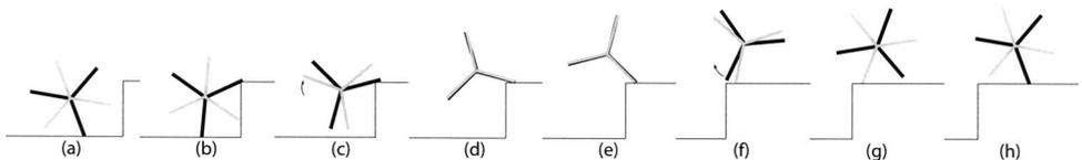
**Figure 2.** Illustration of the Whegs concept. (a) The two front whegs of the robot approach an obstacle; (b) the far (black) whleg makes contact first and (c) while the far whleg is slowed, passive torsional compliance in the drive train allows the near (gray) whleg to rotate into phase with the far whleg; (d) once in phase, the two whegs can (e) propel the front of the robot over the obstacle; (f) atop the obstacle the two whegs separate and (g) spring back to their (h) prior configuration.
