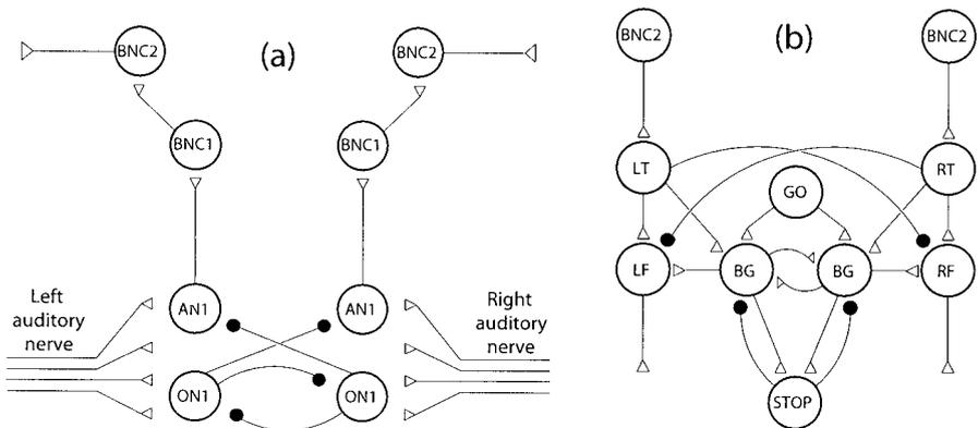
**Figure 3.** Neural circuits based on cricket neurophysiology for (a) auditory processing and (b) motor control. The circuits were simulated in real-time using Whegs ASP’s onboard PC104 computer. The simulation is based on an integrate and fire neural model with conductance-based synapses.
