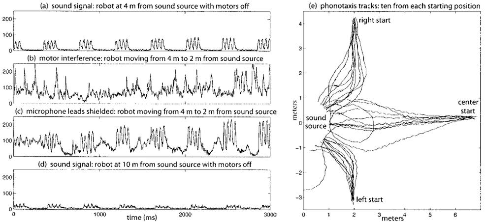
**Figure 5.** (a)–(d) Actual auditory input for outdoor phonotaxis at different distances and with and without electromagnetic and acoustic interference from the drive motor. (e) Thirty consecutive outdoor trials, recorded using the tracker, showing the robot approaching the sound source from different directions.
