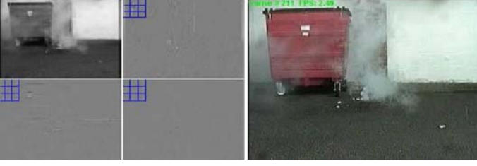
Fig. 1. Image frame with smoke and its single level wavelet subimages. Blurring in the edges is visible. The analysis is carried out in small blocks.
