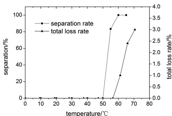
**Figure 3.** Effect of temperature on aluminium–plastic separation and loss.
