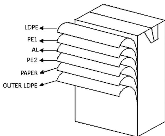
Figure 1. Schematic structure of Tetra Pak.
