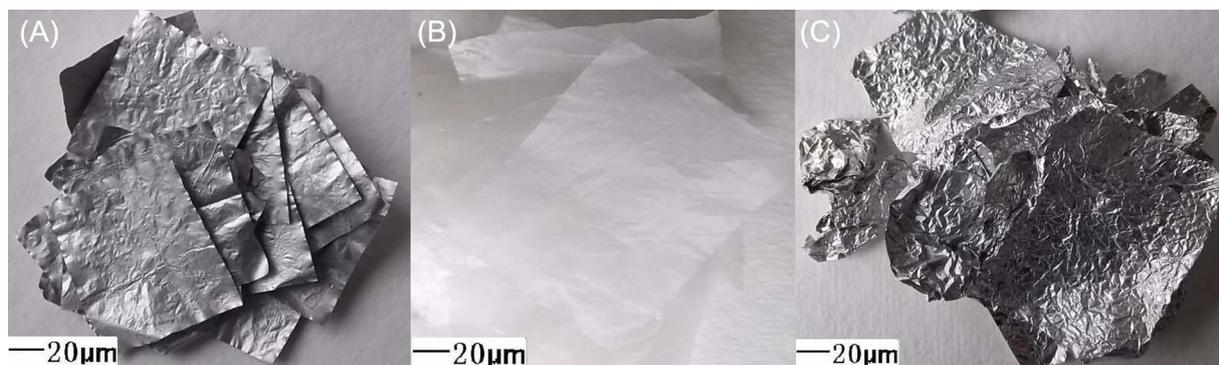
Figure 2. Images of the separated layers: (A) separated Al-PE laminates, (B) separated PE, (C) separated aluminum layer.
