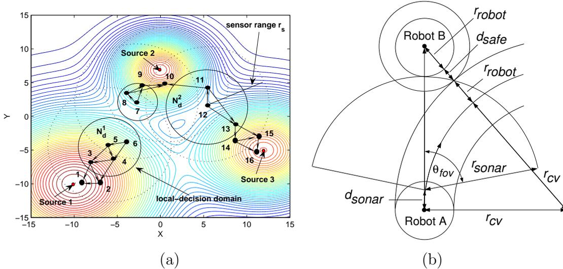
Fig. 1. a) Network architecture resulting from the constraints of communication range  $r_s$  and adaptive decision-range  $r_d^i$  that are imposed on the agents in the GSO algorithm. b) The obstacle avoidance model used by the robots in embodied simulations of the GSO algorithm.
