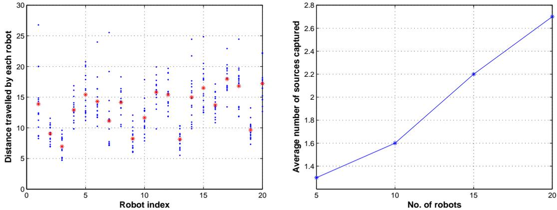
Fig. 6. a) Distance travelled by each robot over 15 trials where the same initial placement is used. b) Performance across group size: Average number of sources captures in a set of 10 experimental trials
