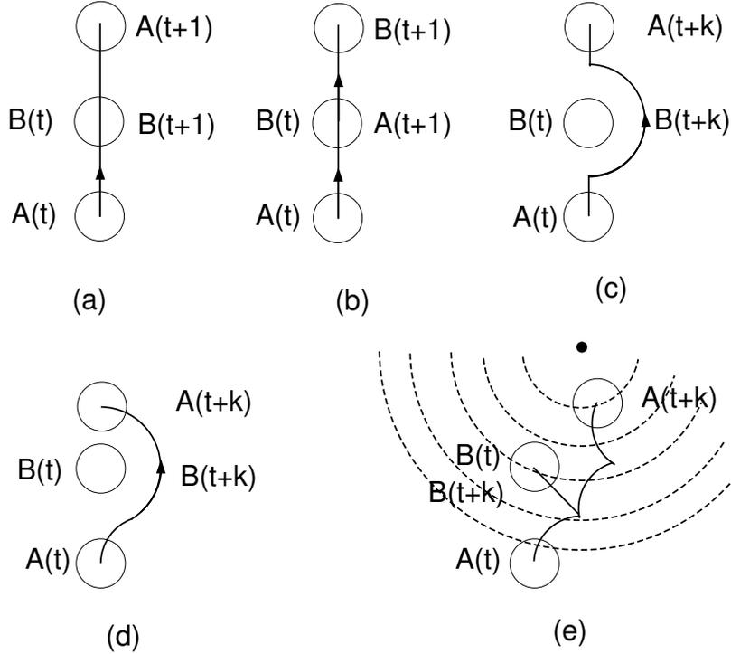
Fig. 2. a) Leapfrogging behavior according to the GSO algorithm. b), c), and d) Three methods of robotic implementation of explicit leapfrogging behavior. e) Implicit leapfrogging behavior due to obstacle avoidance.
