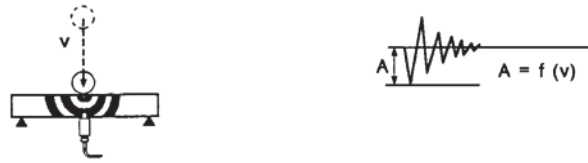
Fig.3.1. Scheme of a ball shock on a plate, amplitude A of a pressure wave and a signal
