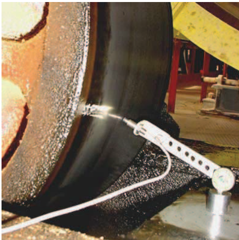
Fig.3.2. Measurement of shaft vibration and radial shaft displacement with proximity probes
