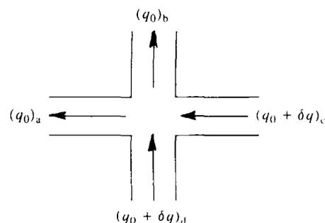
Fig. 3. Shear flow at a typical node
