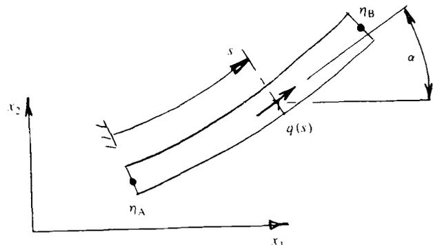
Fig. 2. Shear flow in a limb
