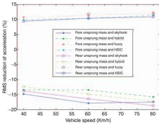
Figure 23. The vibration acceleration reduction comparison of fore or rear suspension unsprung mass on D class road.
