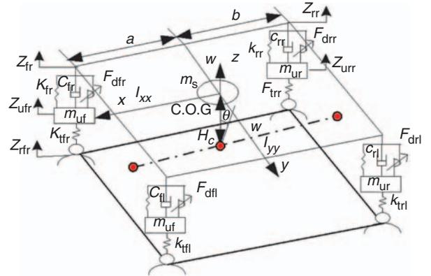
Figure 5. Mechanical model of the MR suspension system.
