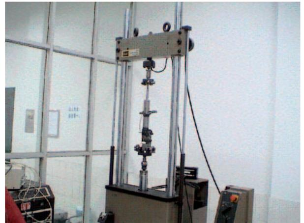
**Figure 2.** MTS material testing system.
