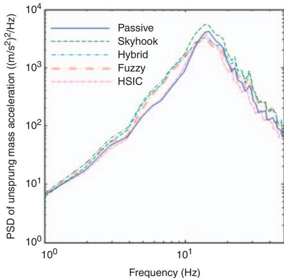
**Figure 19.** The PSD of unsprung mass acceleration under bump input at vehicle speed of 80 km/h on B class road.
