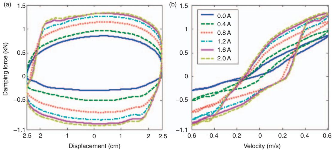
Figure 3. Plots for damping force vs displacement and for damping force vs. velocity at peak velocity of 0.6 m/s.
