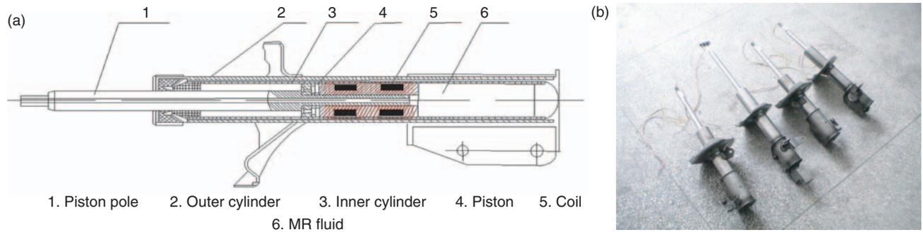
**Figure 1.** The MR dampers of a passenger vehicle: (a) schematic configuration, (b) photograph of four MR dampers.
