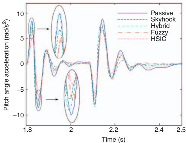
Figure 17. The pitch angular acceleration time history of body under bump input at vehicle speed of 30 km/h.
