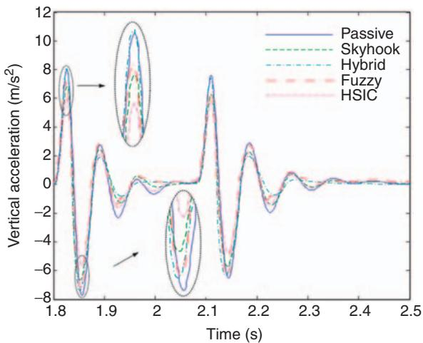
Figure 16. The time history of vertical acceleration of body under bump input at vehicle speed of 30 km/h.
