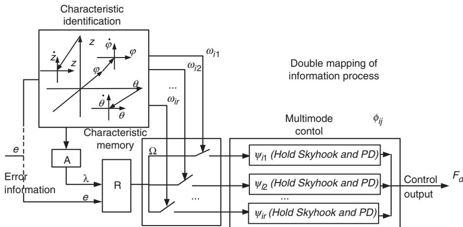
Figure 8. Double mapping relation of HSIC in control and decision.
