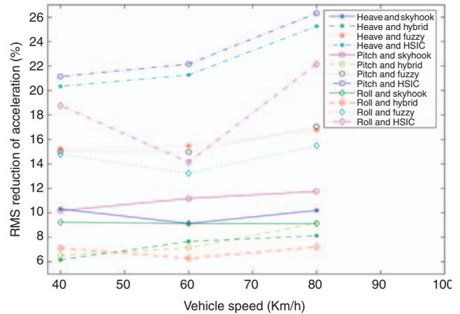
**Figure 20.** The vibration acceleration reduction comparison of vehicle body on B class road.
