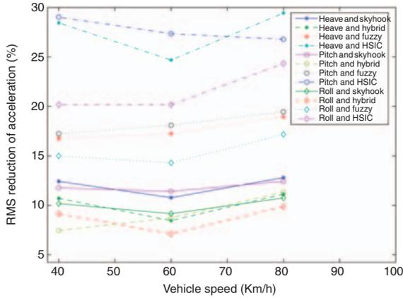
Figure 22. The vibration reduction acceleration comparison of vehicle body on D class road.
