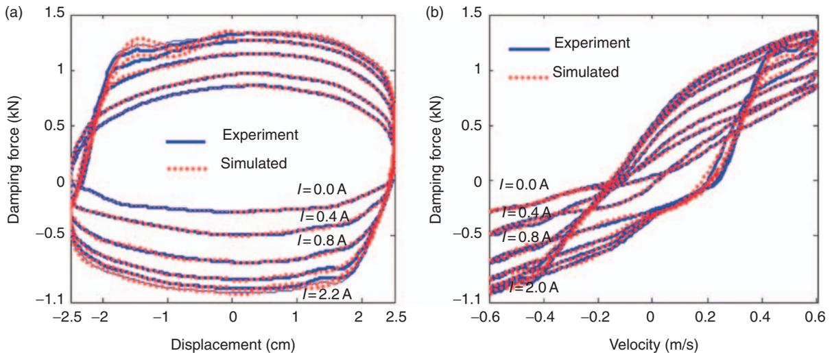
Figure 4. Comparison of polynomial model and experimental results (3.8197 Hz, 25 mm): (a) force vs displacement; (b) force vs velocity.
