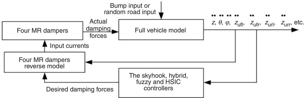
**Figure 13. Block diagram of semi-active controllers for full vehicle suspension model with four MR dampers.**
