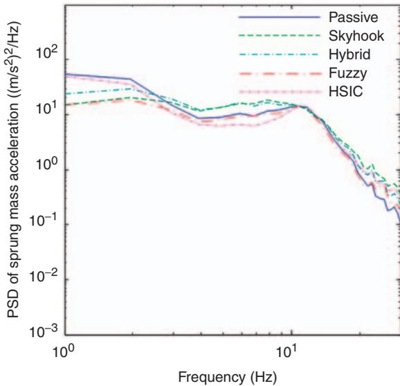
**Figure 18.** The PSD of sprung mass acceleration under bump input at vehicle speed of 80 km/h on B class road.
