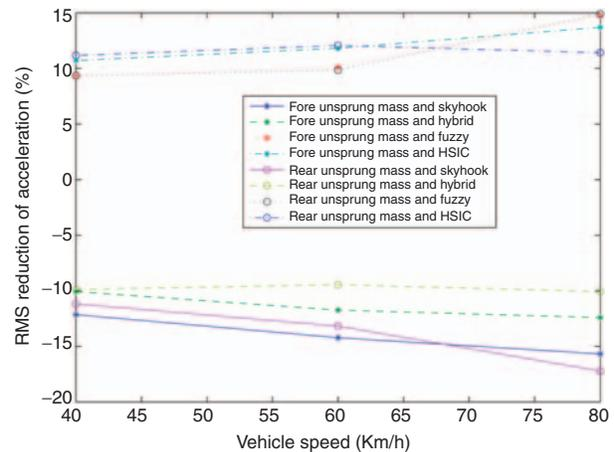
**Figure 21.** The vibration acceleration reduction comparison of fore or rear suspension unsprung mass on B class road.
