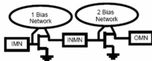
Fig. 2 Two-stage Power Amplifier Topology
