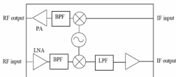
Fig. 1 Transceiver Diagram
