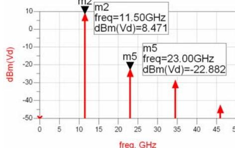
Fig. 6 Harmonics Spectrum
