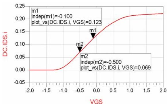
Fig. 3 Transconductance Characteristics
