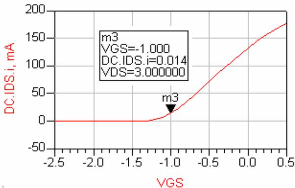
Fig. 9 Transconductance Characteristics
