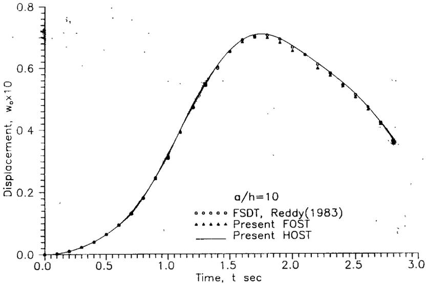
**Figure 5a.** Displacement vs. time for a simply supported (S2) square cross-ply ( $0^\circ/90^\circ$ ) laminated plate under suddenly applied uniform pulse load ( $q_0 = 0.005$ ,  $\Delta t = 0.01$  sec).
