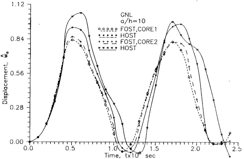
Figure 6b. Displacement vs. time for a clamped (C) angle-ply sandwich ( $0^\circ/45^\circ/90^\circ/\text{CORE}/90^\circ/45^\circ/30^\circ/0^\circ$ ) laminate under suddenly applied uniform transverse load ( $q_0 = 5000 \text{ N/cm}^2$ ,  $\Delta t = 5 \mu\text{sec}$ ).
