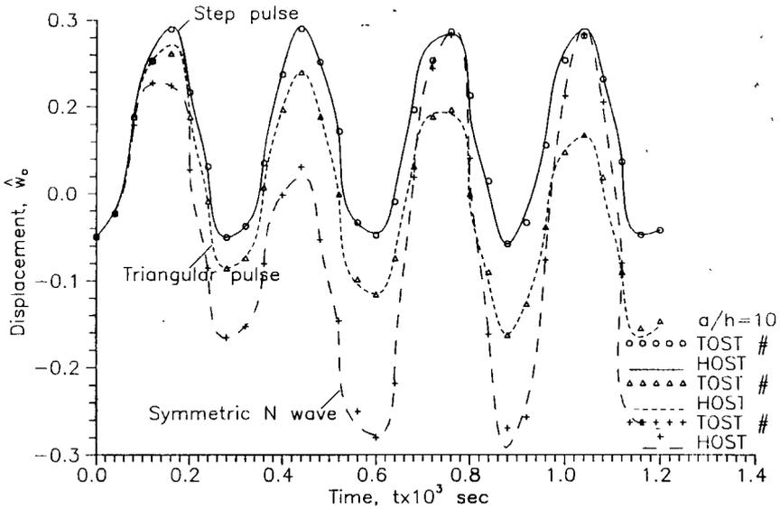
**Figure 3.** Displacement vs. time for a simply supported (S1) square orthotropic three-layer plate ( $q_0 = 4500$  psi,  $\Delta t = 1$   $\mu$ sec).
