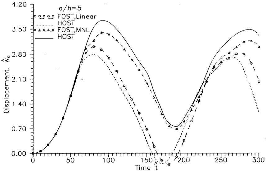
**Figure 8.** Displacement vs. time for a clamped (C) angle-ply ( $45^\circ/ -45^\circ$ ) laminate under suddenly applied uniformly distributed transverse load ( $\Delta t = 0.5 \mu\text{sec}$ ,  $q_0 = 0.9375$ ).
