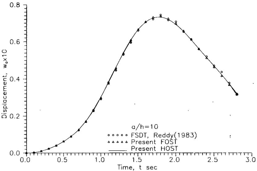
**Figure 5b.** Displacement vs. time for a simply supported (S2) square angle-ply ( $45^\circ/-45^\circ$ ) laminated plate under suddenly applied uniform pulse load ( $q_0 = 0.005$ ,  $\Delta t = 0.01$  sec).
