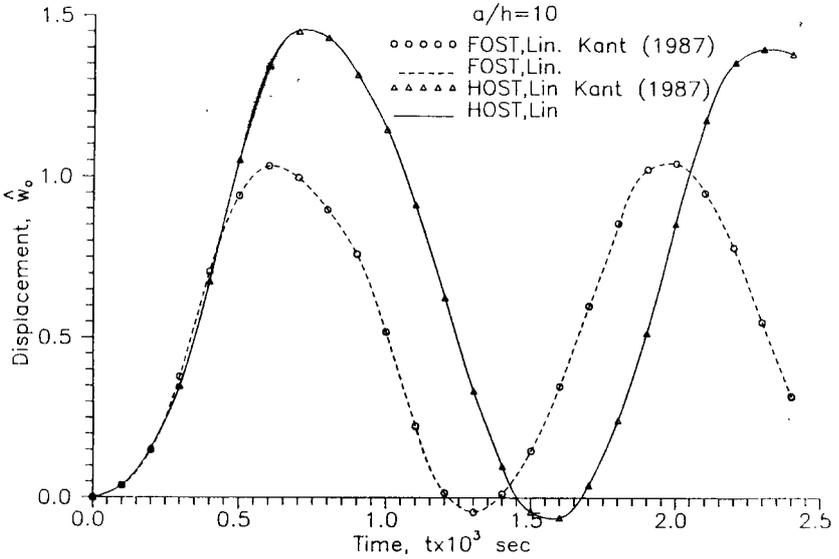
Figure 6a. Displacement vs. time for a clamped (C) angle-ply sandwich ( $0^\circ/45^\circ/90^\circ/\text{CORE}/90^\circ/45^\circ/30^\circ/0^\circ$ ) laminate under suddenly applied uniform transverse load ( $q_0 = 5000 \text{ N/cm}^2$ ,  $\Delta t = 5 \mu\text{sec}$ ).
