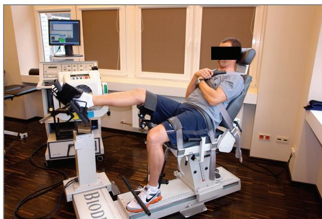
Fig. 1. The measurement of IT using Biodex System 3
