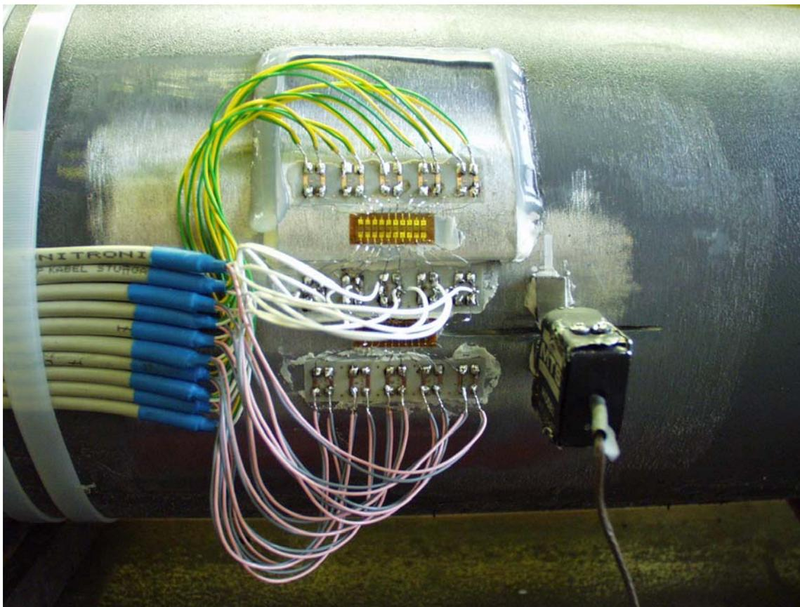
Figure 1. Pipeline section (*B\_b8*) with artificial longitudinal gouge, strain-gages and an extensometer
