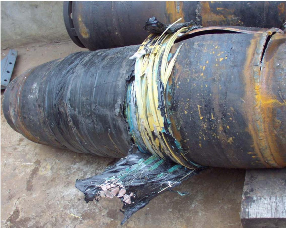
Figure 4. Externally reinforced pipeline section (girth weld) *CS\_a1* after the burst test
