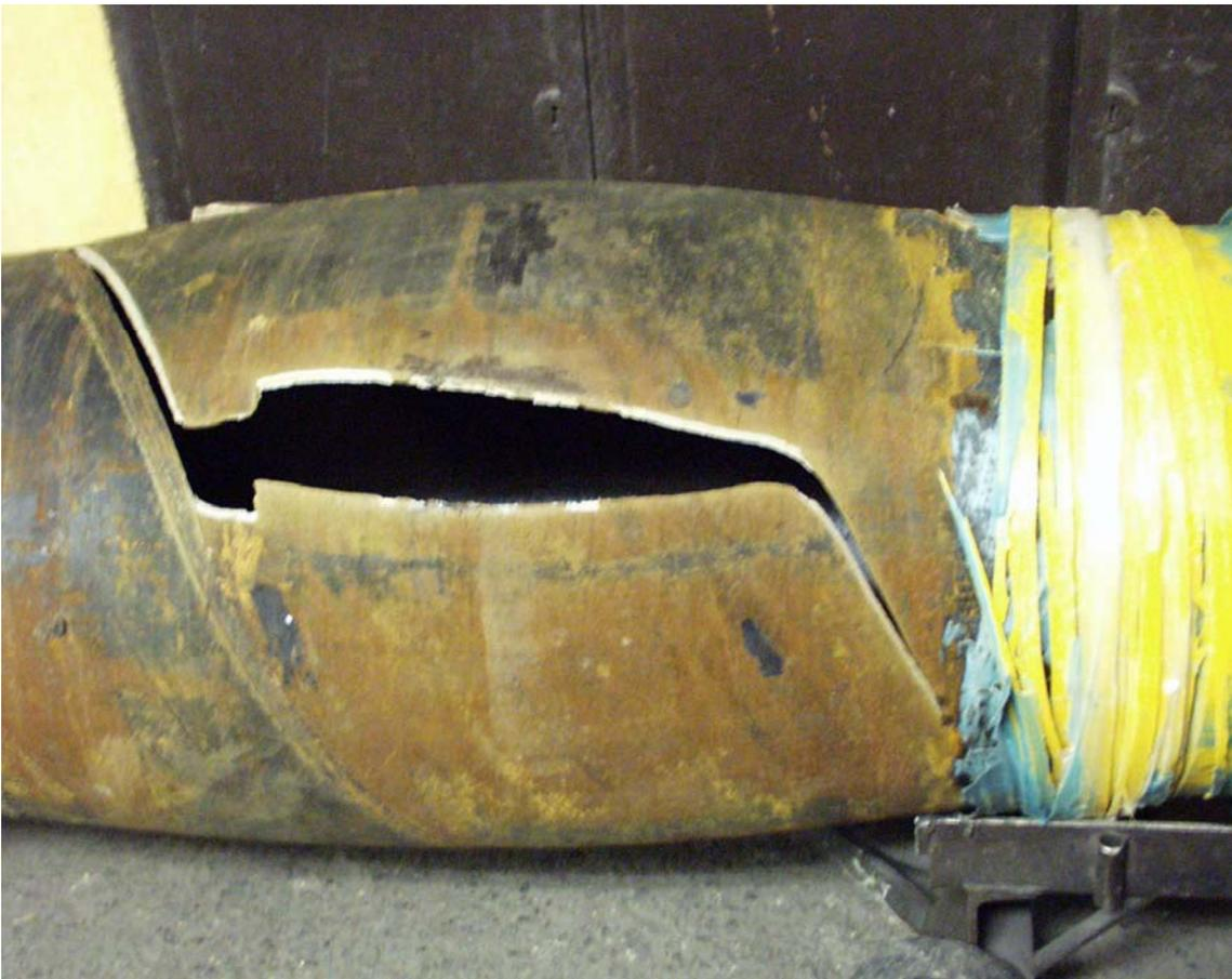
Figure 6. The failed area of the externally reinforced pipeline section (girth weld) *CS\_b3* after the burst test
