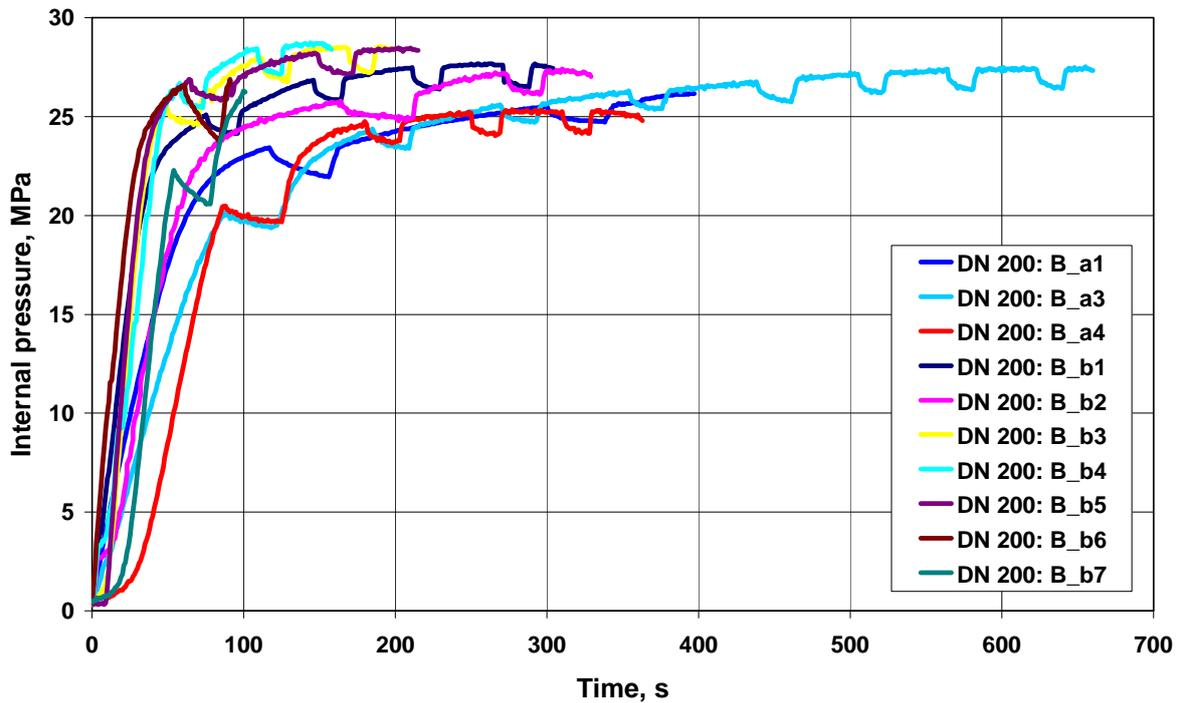
Figure 2. Internal pressure vs. time diagrams during the burst tests of the pipeline sections in the  $B_a$  and the  $B_b$  testing groups
