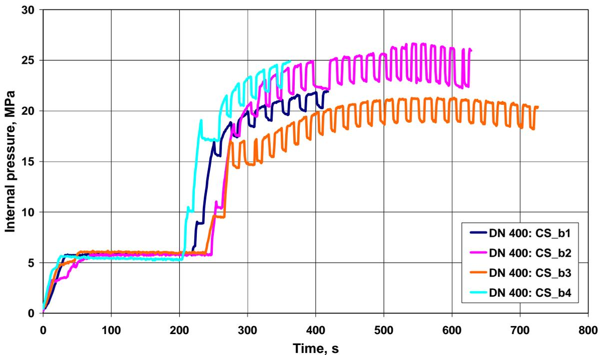
Figure 2. Internal pressure vs. time diagrams during the burst tests of the pipeline sections in the  $CS_b$  testing group
