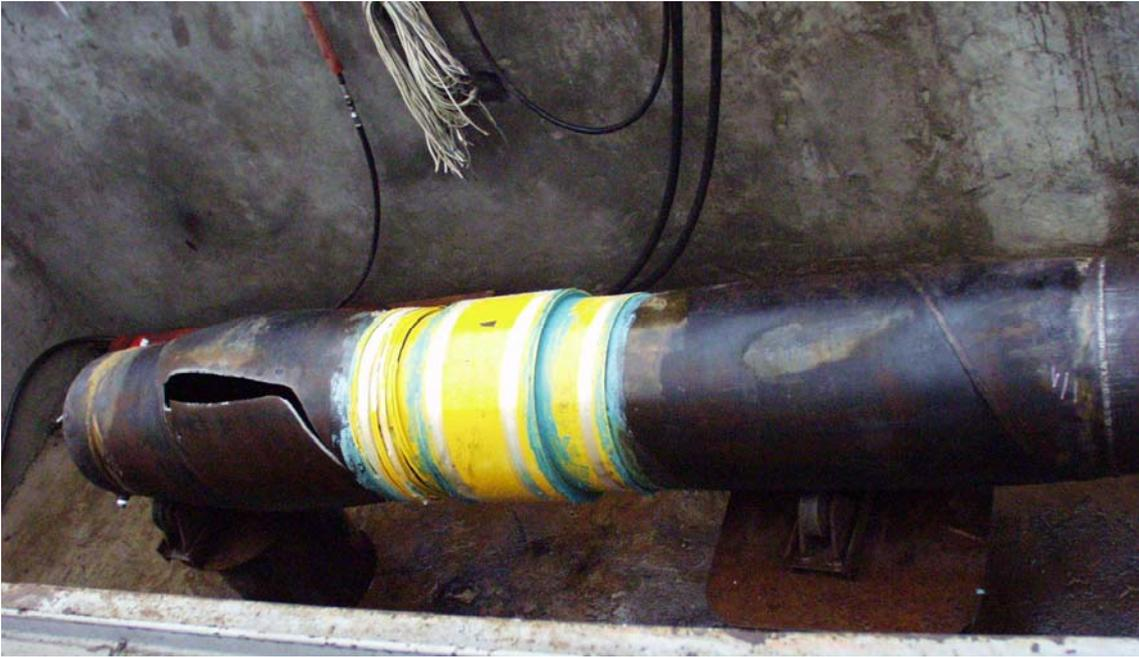
Figure 5. Externally reinforced pipeline section (girth weld) *CS\_b3* after the burst test
