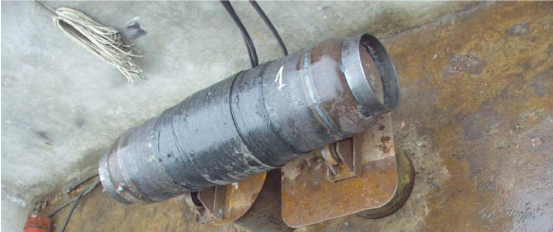
Figure 3. Externally reinforced pipeline section (girth weld) *CS\_a1* before the burst test
