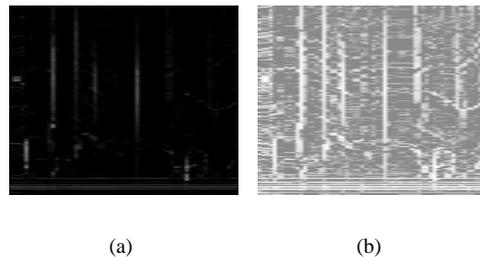
FIG. 5: White top-hat filtering: (a) result of the white top-hat and (b) result of the histogram equalization of (a).
