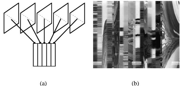
FIG. 2: Video transformation: (a) simplification of the video content by transformation of each frame into a column on the visual rhythm representation; (b) a real example considering the principal diagonal sub-sampling.
