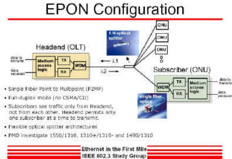
Figure 6 Ethernet Passive Optical Network [6]
