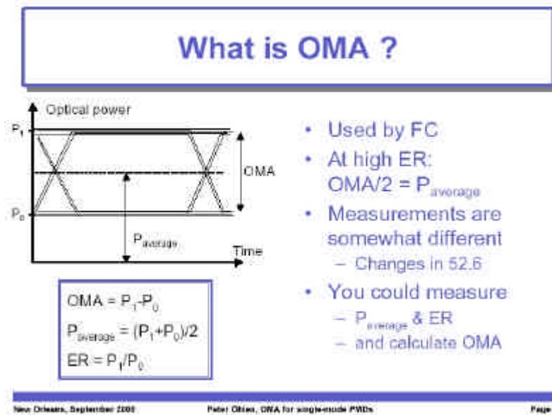
Figure 2 Optical Modulation Amplitude [2]
