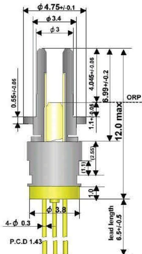
**Figure 5 TOSA drawing example: NEC [6]**
