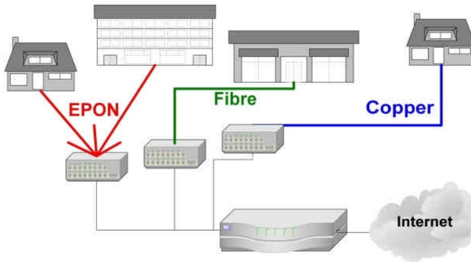
**Figure 1 The three EFM access methods [1]**
