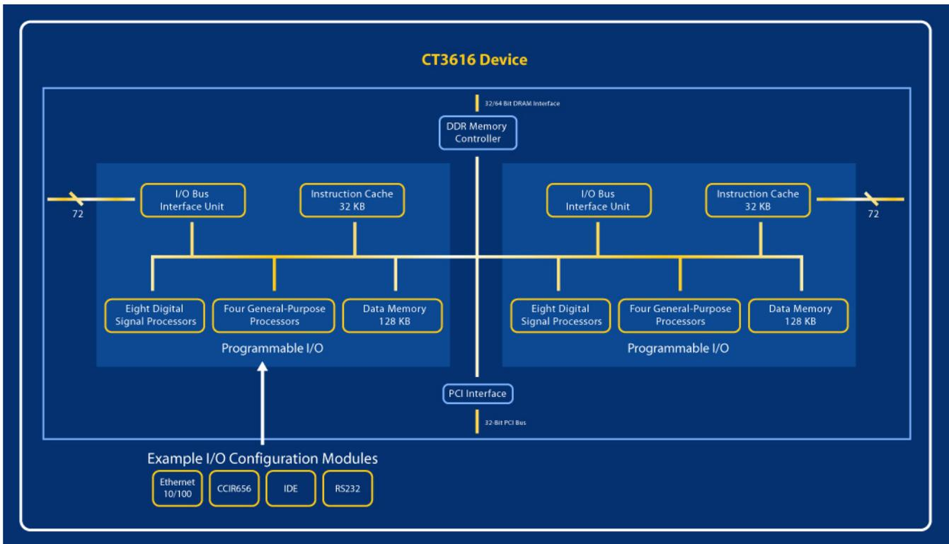
**Figure 3: Compute Engine: CT3616 block diagram**
