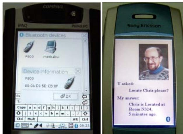
Fig. 3. Snapshot Bluetooth access point on PDA and user client on Mobile Phone PDA
