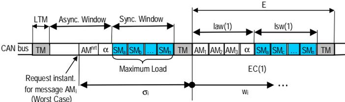
**Figure 2** – Combining event-triggered and time-triggered traffic in FTT-CAN
