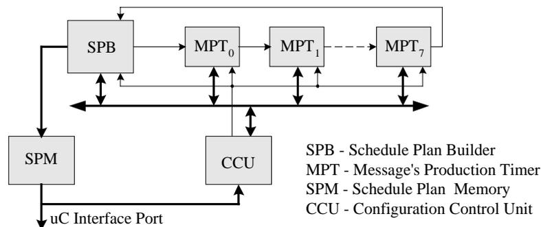
**Figure 3** – Architecture of PSCoP scheduling co-processor
