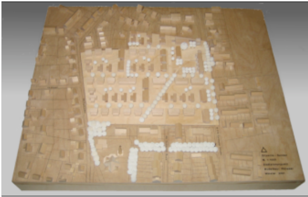
Figure 2. Example section of a city development plan within cadastral information (left) and a corresponding physical block model made of wood downscaled to 1:1000 (right)
