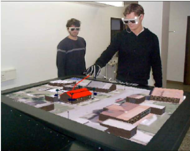
Figure 4. Virtual 3D city model and improved virtual pointer. The image has been manipulated to illustrate the stereoscopic effect
