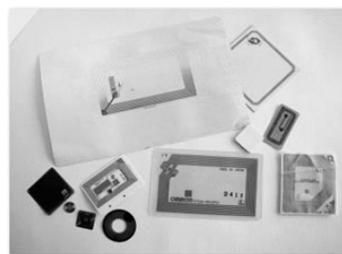
Fig 5 Variety of RFID Tag Formats
