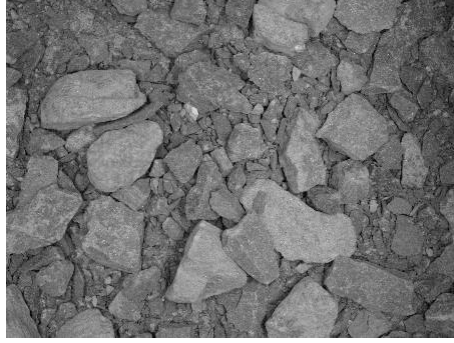
Fig. 1. An image of construction aggregate. The properties of the aggregate are defined by size for larger pieces, and by granularity for finer pieces.
