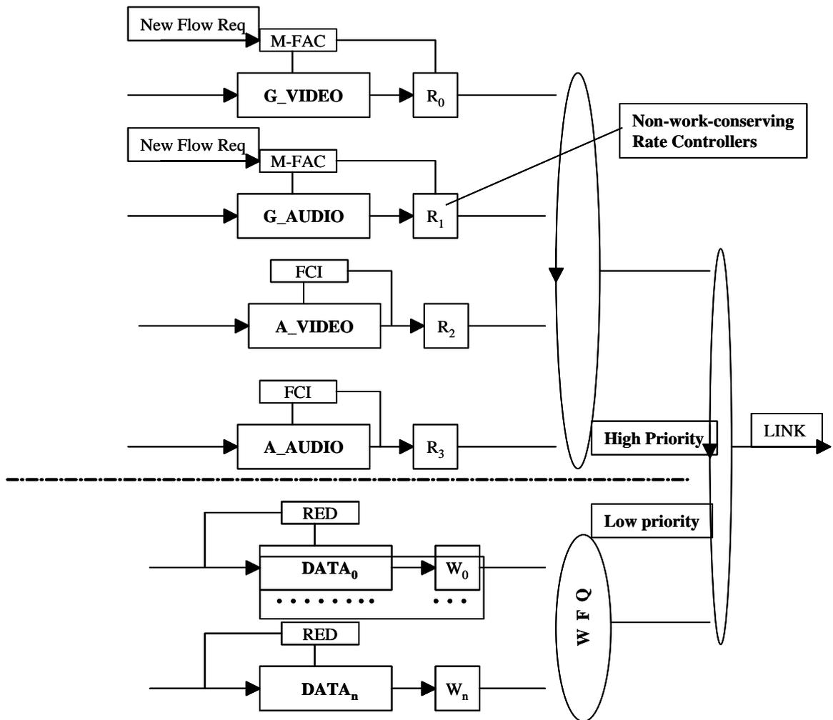
**Fig. 2 Bandwidth Sharing and Resource Control Model.**
