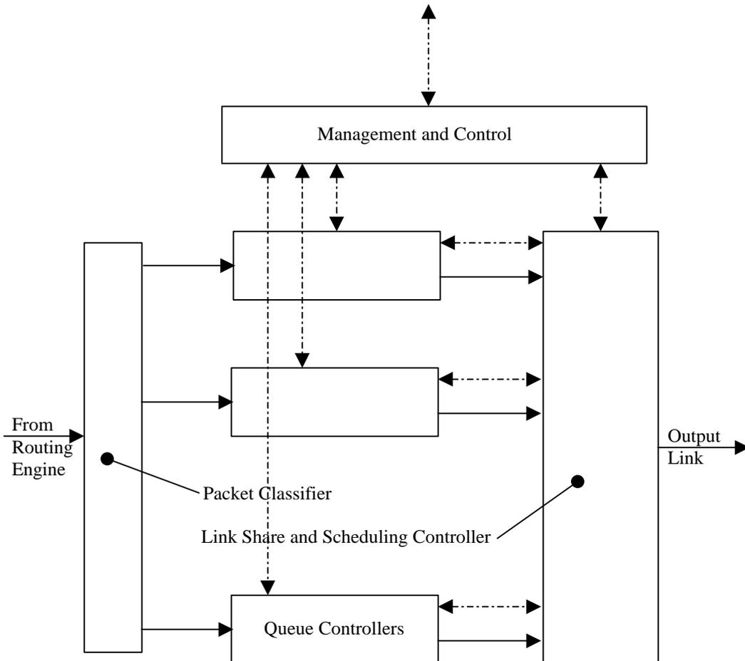
**Fig. 4 Link Share Controller Architecture**
