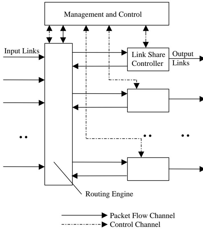
**Fig. 3 General Architecture of the Router**
