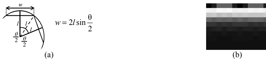
Figure 3. (a) As the SE of length l is rotated by \theta , w should be such that the edges of this SE touch when rotated. (b) A Scale-Orientation Pixel Signature generated with the new method, taken from the centre of a Gaussian blob (note the improved structure over that in Figure 1 (a)).
