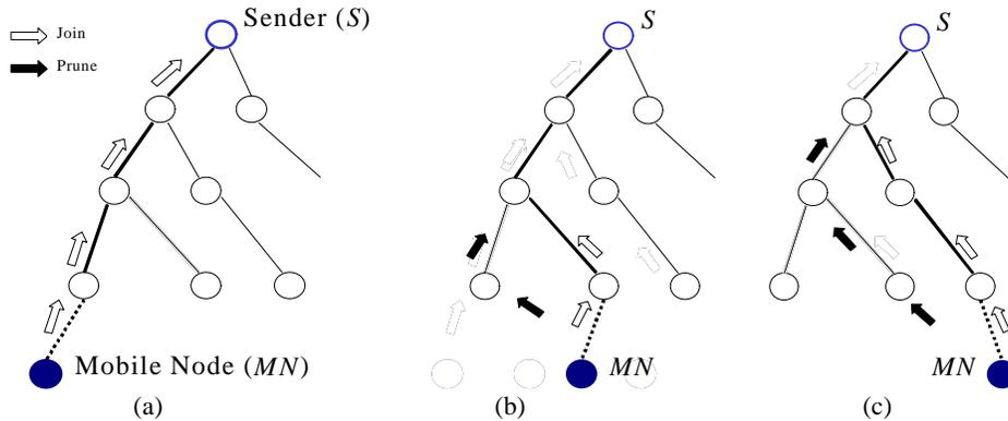
Figure 6. Multicast-based mobility. As the MN moves, as in (b) and (c), the MN joins the distribution tree through the new location and prunes through the old location.
