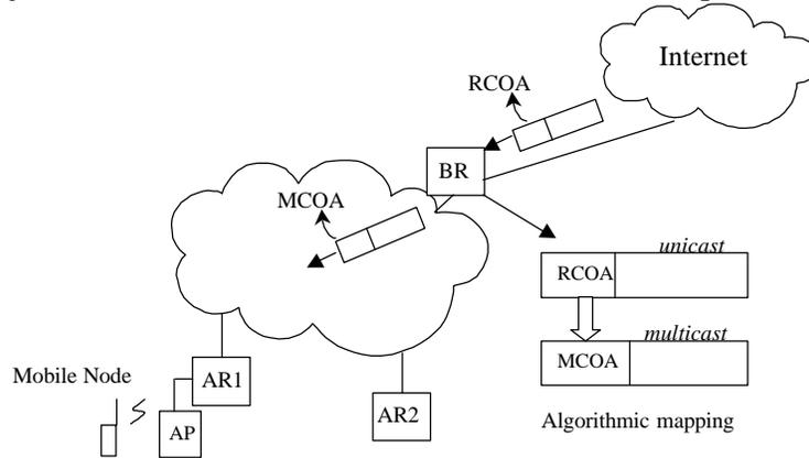
Figure 7. High level architectural view: Data packet is unicast over the Internet destined to the RCOA and arrives at the border router (BR) for the mobile node. The BR intercepts the packet and performs algorithmic mapping from the RCOA to MCOA. The packet is then multicast within the domain to the mobile node.
