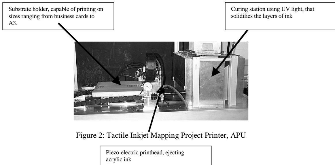
Figure 2: Tactile Inkjet Mapping Project Printer, APU
