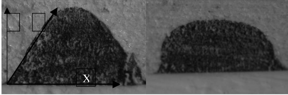
Figure 7a and b: left to right, Normal line and line printed using SDP. 360 dpi
