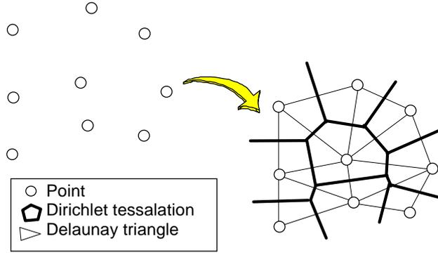
Figure 4. Dirichlet tessellation and Delaunay triangulation of a Finite point set.
