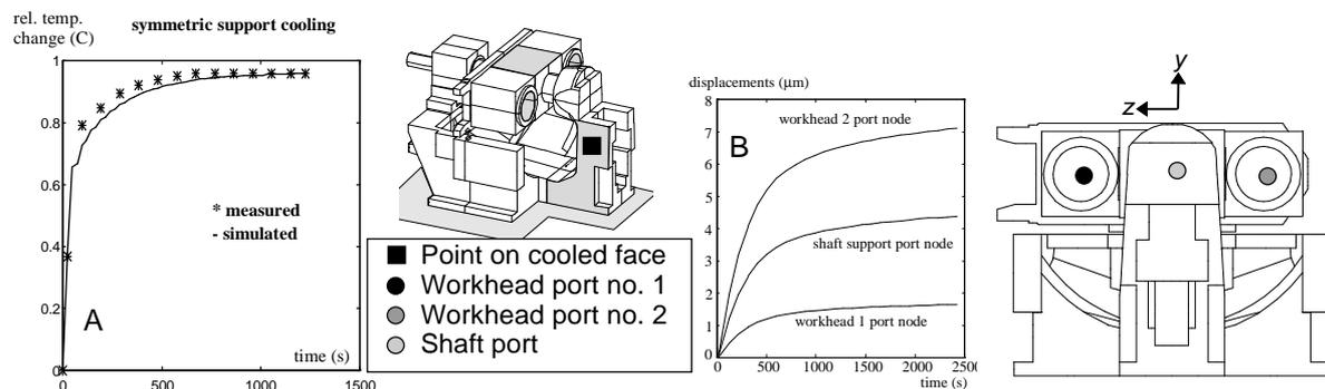
Figure 12. Simulated and measured effect of a cooling temperature step change in A, and workhead thermoelastic movements in B.
