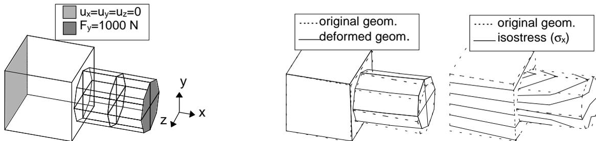
Figure 8. Loading and boundary condition, deformed shape, and bending stress.
