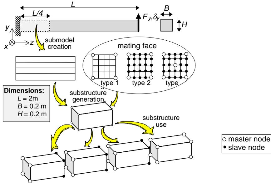
Figure 9. A substructuring example.
