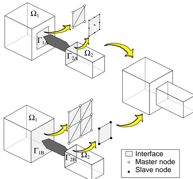
Figure 3. Master-slave relationship between geometrically compatible/incompatible faces.
