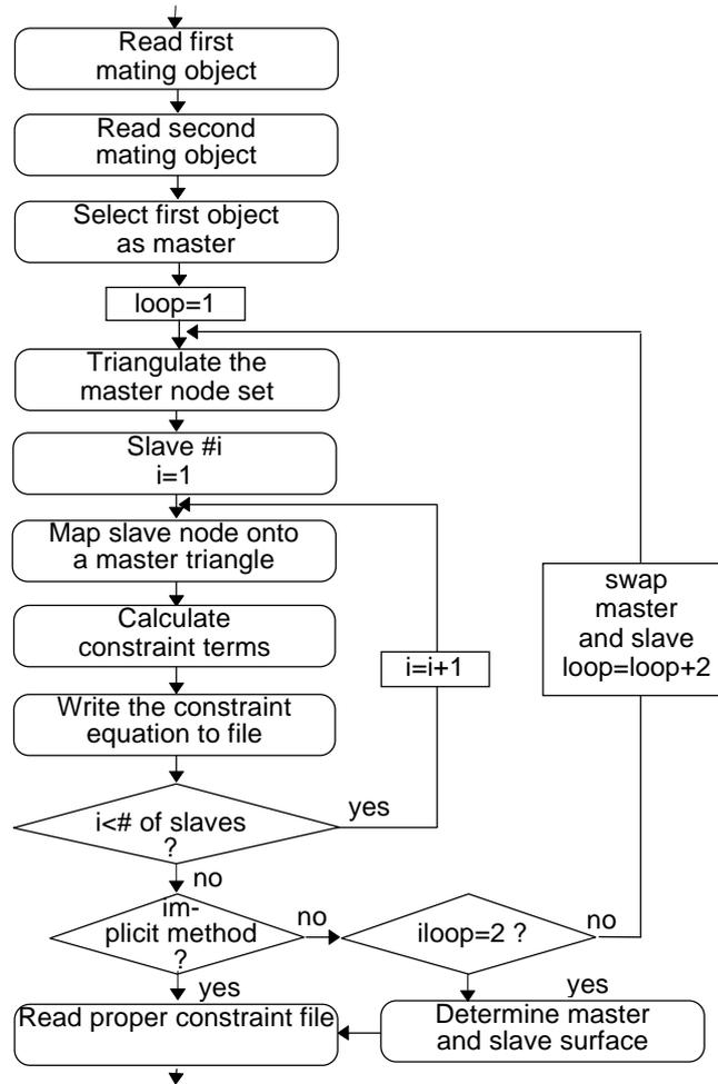
Figure 2. Logic for identifying and constraining slave DOFs.
