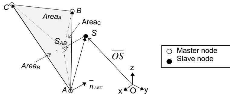
Figure 6. Master triangle and sub-triangles required for the constraint terms.
