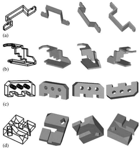
Fig. 12. Reconstruction results 2 (leftmost: sketch drawings, right 3: the reconstruction results in rendering): (a) Sheet metal, (b) General mechanical part, (c) Product with hole, and (d) General product with hole.
