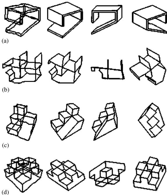
Fig. 11. Reconstruction results 1 (leftmost: sketch drawings, right 3: the reconstruction results in wireframe): (a) Manifold object (orthogonal), (b) Non-manifold object (parallel or freehand), (c) Manifold object (perspective), and (d) Object with hole (perspective).
