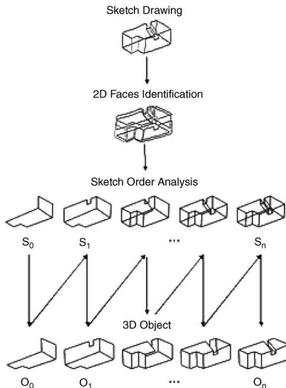
Fig. 2. Overview of the progressive 3D reconstruction.
