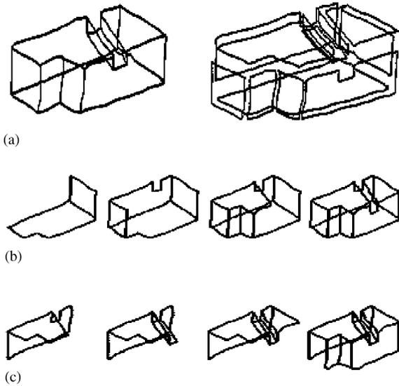
Fig. 5. Sketch order analysis: (a) Off-line sketch drawing and face identification, (b) Normal sketch order, and (c) Abnormal sketch order.
