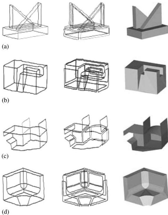
Fig. 13. Experimental results (left: input 2D sketches, center: identified 2D faces, right: reconstructed 3D object): (a) Polyhedral object, (b) Manifold polyhedral object, (c) Non-manifold curvilinear object (sheet metal), and (d) Curvilinear object with conical, spherical and cylindrical surfaces.
