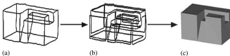
Fig. 1. Conceptual design with sketching: (a) Sketch drawing, (b) 2D identified faces, and (c) 3D object.
