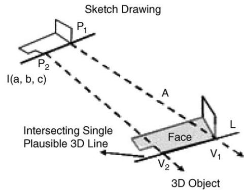
Fig. 8. Face constraint.
