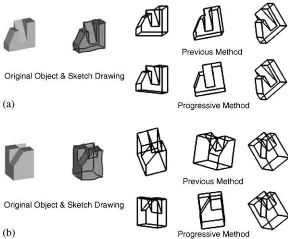
Fig. 15. The accuracy comparison of practical objects between Lipson [8] and ours: (a) Practical object 1, and (b) Practical object 2.
