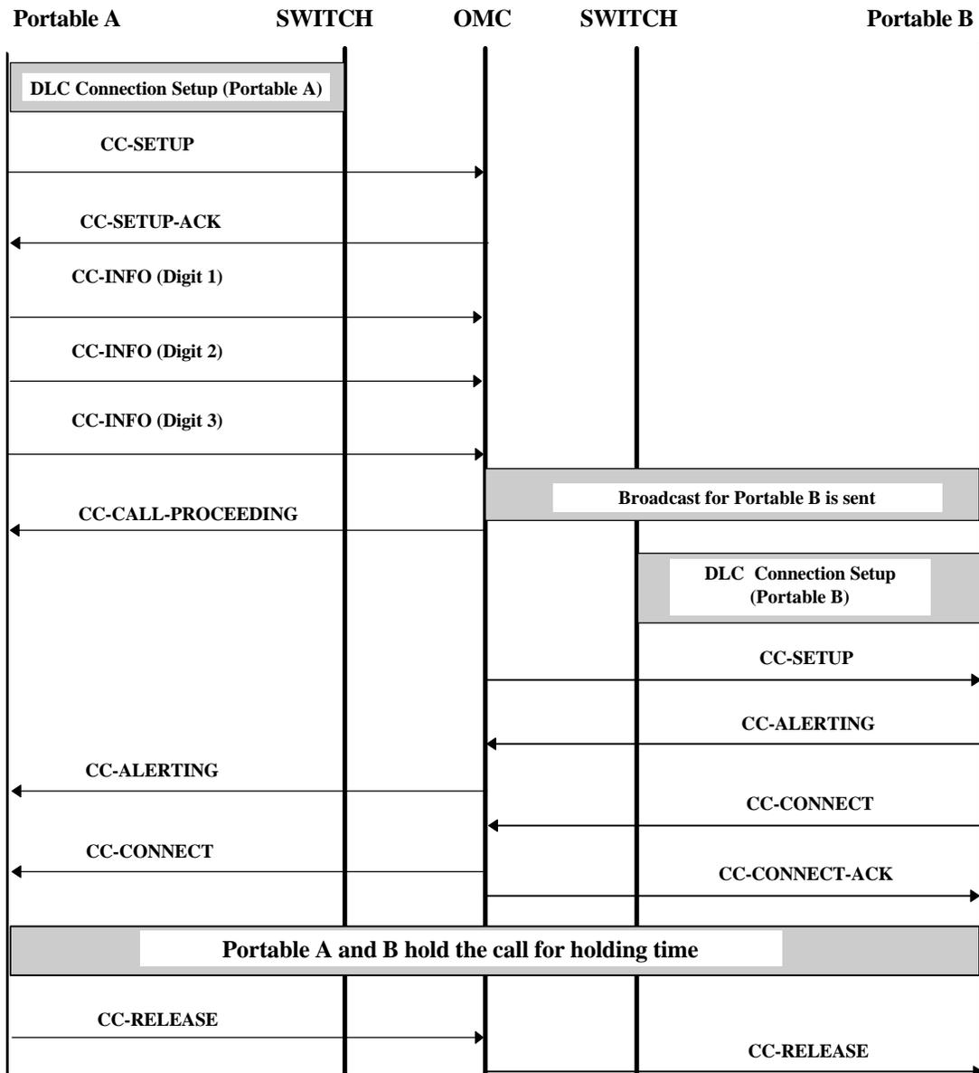
Fig. 3 Network Layer messages exchanged for one complete call
