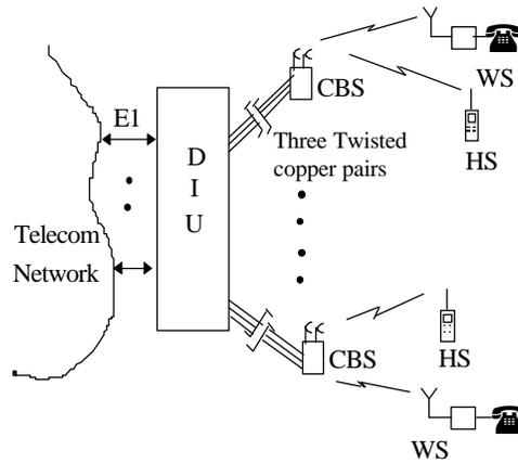
Fig. 1 1,000-line corDECT system architecture
