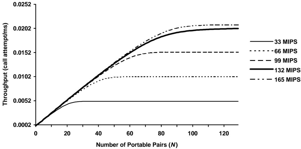
Fig. 11 Comparison of the throughput characteristic for various MIPS at SWITCH
