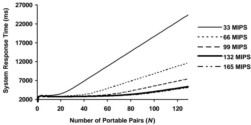
Fig. 10 Comparison of the response time characteristic of system for varying MIPS at SWITCH server
