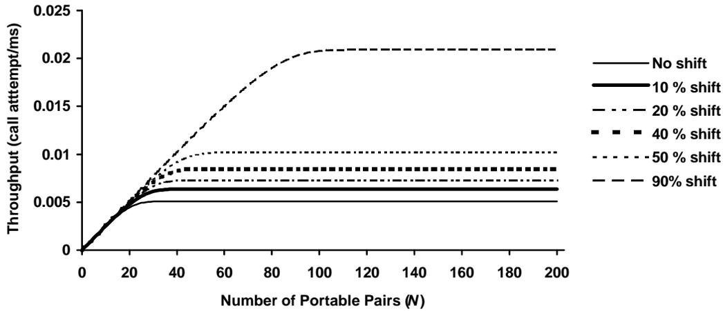
Fig. 13 Comparison of throughput characteristic for different percentage of shift of SWITCH server demand to BIM server
