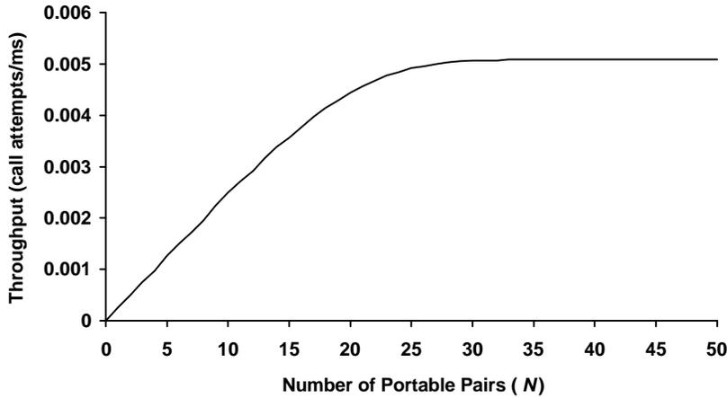
Fig. 6 System throughput characteristic from analytical model for varying  $N$ . (At the Saturation Value,  $N = 30$ , Throughput = 0.005 call attempts/ms).
