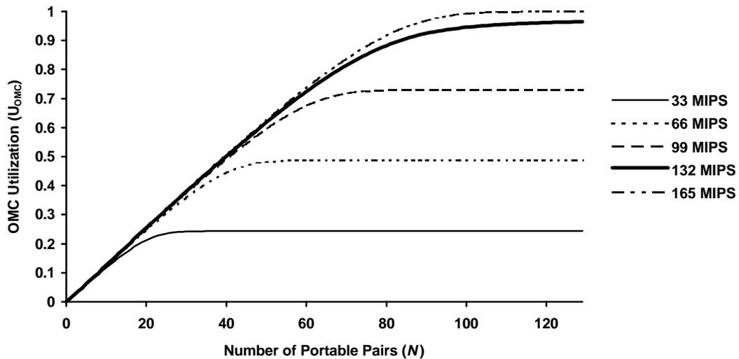
Fig. 9 Comparison of the utilization characteristic of OMC server for varying MIPS at SWITCH server
