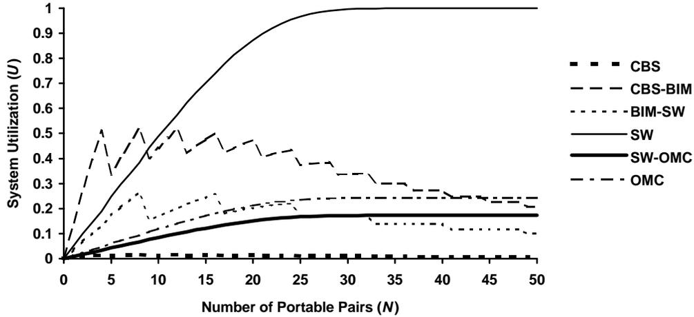
Fig. 7 System utilization characteristic from analytical model for all servers in corDECT system for varying  $N$ .
