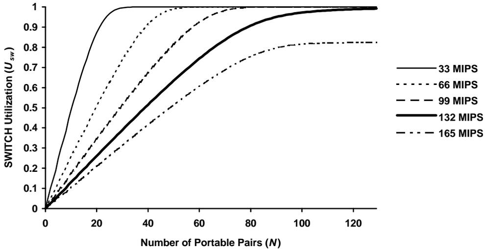
Fig. 8 Comparison of utilization characteristic for various MIPS at SWITCH server
