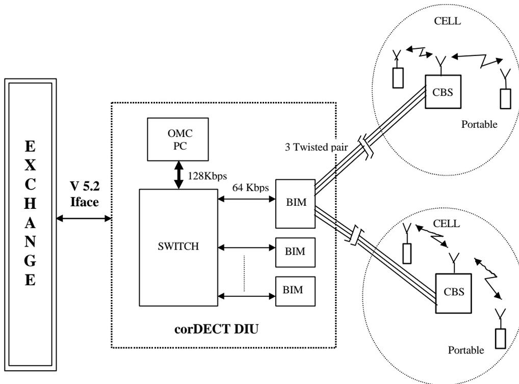
Fig. 2.2 corDECT 1000-line system architecture
